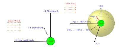
**Figure 1.** Code coordinates scheme (left) and spherical coordinates illustration used in MP derivation (right)
