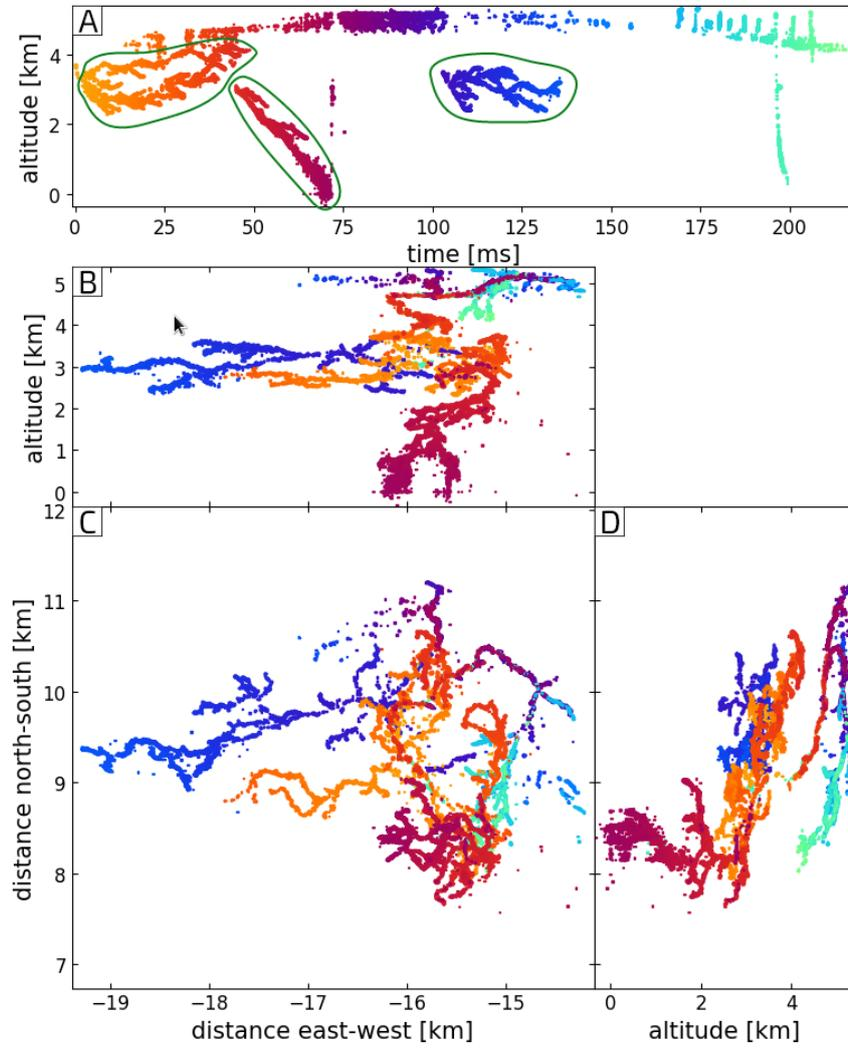
**Figure 1.** Plan view of the imaged data, coloured by time. Each point represents a located VHF source. Negative leaders are circled in green. A) Time vs altitude (from ground). B) east-west distance (from core center) vs altitude. C) east-west distance (from core center) vs north-south (from core center). D) altitude (from ground) vs east-west distance (from core center).
