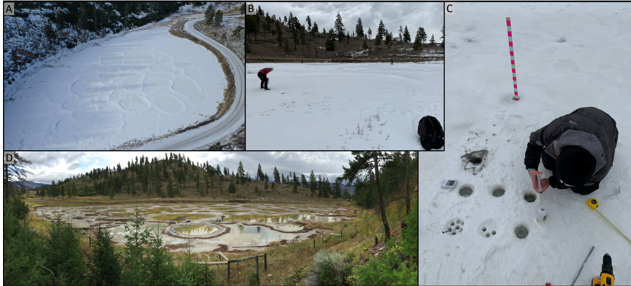
Figure 4 – Field work at Basque Lake 2. A) Drone image of Basque Lake 2 taken in February 2019. The segregated brine pools, more evident in (D), can still be seen under the snow cover. B) Ground photo of a sample site as we begin to drill the borehole array seen in the next panel. C) The typical sampling procedure where ice thickness and temperature are recorded, ice cores are gathered, and brine is extracted from the underlying lake. D) The lake without an ice cover, photographed in September 2019 (taken from hillside at top left of image A).
