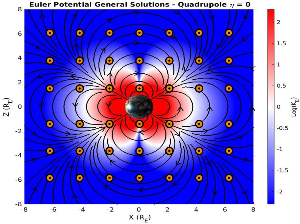
**Figure A.** General solutions for the Euler potentials. Black streamlines correspond to the  $\vec{E} \times \vec{B}$  Euler potentials, and the orange vectors pointing out of the figure are the  $\vec{E}$  Euler potentials. Colormap indicates the dominant electric field. Note the similarity of the  $\vec{E} \times \vec{B}$  and  $\vec{E}$  streamlines to those illustrated in Figure 3.
