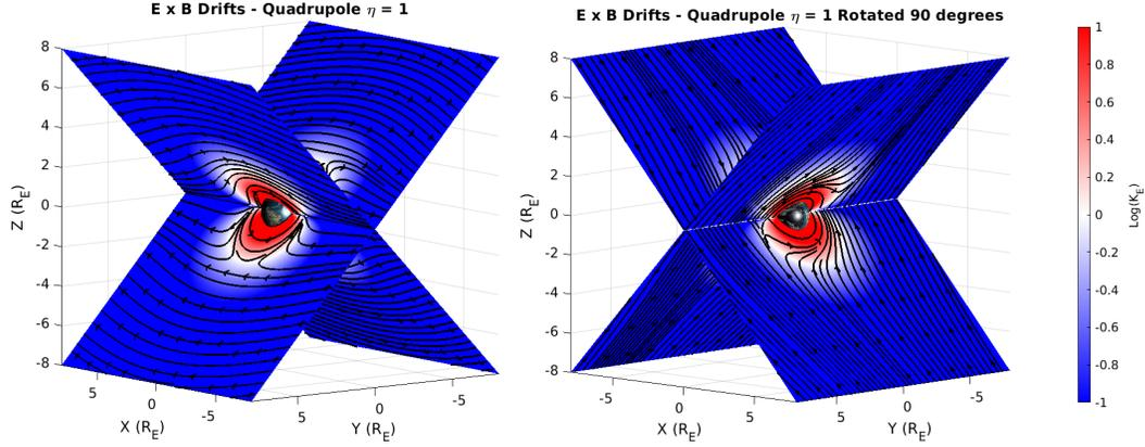
**Figure 5.** (Left)  $\vec{E} \times \vec{B}$  streamlines along the magnetic equators for  $\eta = 1$ . The colors denote whether the region is on a corotation or convection field dominated region. (Right)  $\vec{E} \times \vec{B}$  streamlines for the  $\eta = 1$  magnetic field 6 hours later. Note the decrease of corotational domination where the equatorial surfaces converge.
