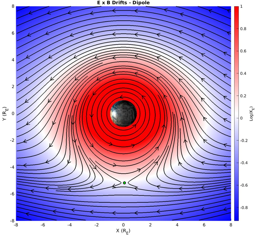
**Figure 2.** The  $\vec{E} \times \vec{B}$  drift field streamlines around Earth on the magnetic/geographic equator. All space that is red is dominated by the Corotational E-Field, and all space in blue is Convection E-Field dominated. The green dot is the location of the stagnation point.
