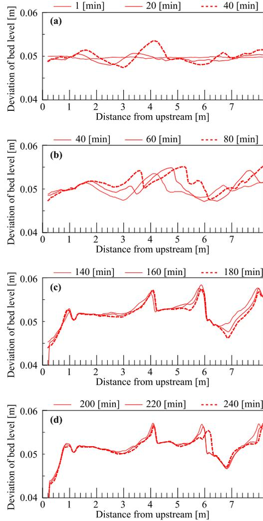
**Figure 4.** Longitudinal view of the measured bed shape. (a) Initial stage of the experiment, (b) occurrence of the alternate bars, (c) intermediate stage of the experiment, and (d) the final stage of the experiment
