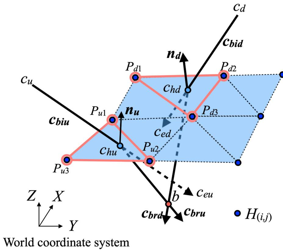
**Figure A5.** Outline of the bed surface measurement method while considering the refraction on the water surface
