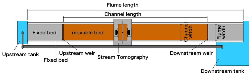
**Figure 2.** Plan view of the experiment flume
