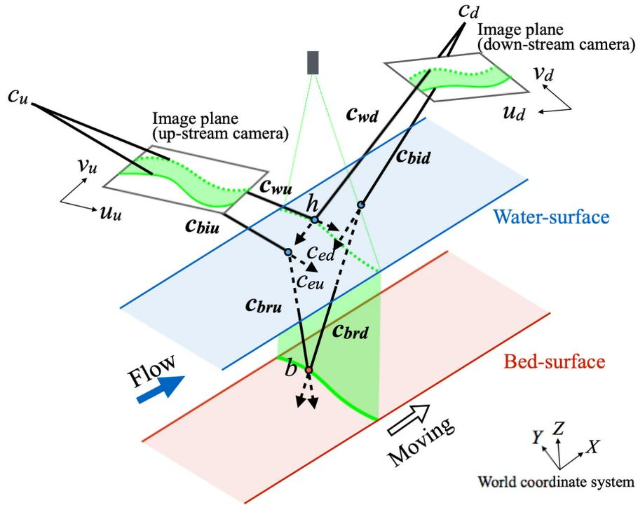
**Figure A3.** Outline of the measurement principle of the water surface and bed surface by triangulation
