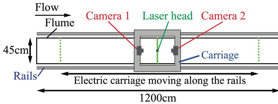
**Figure A1.** Overall plan view of the measurement device
