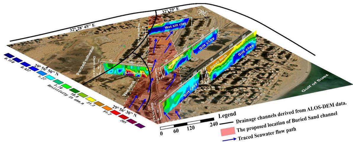
**Fig. 7** shows the existence of the buried sand drainage channel passes from the western part of profile P1 through the top eastern part of profile P7 and western profile P5, going toward the western portion of profile P6.
