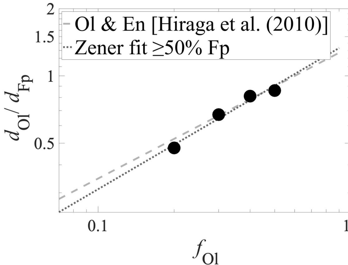
Ratio of grain sizes versus fraction of Ol for samples containing  $\geq 50\%$  Fp fit using the Zener relation. This fit yields  $m = 0.66$  indicating secondary phase grains are small relative to the primary phase and occur along grain boundaries or are randomly distributed throughout the matrix [Evans et al. (2001)].
