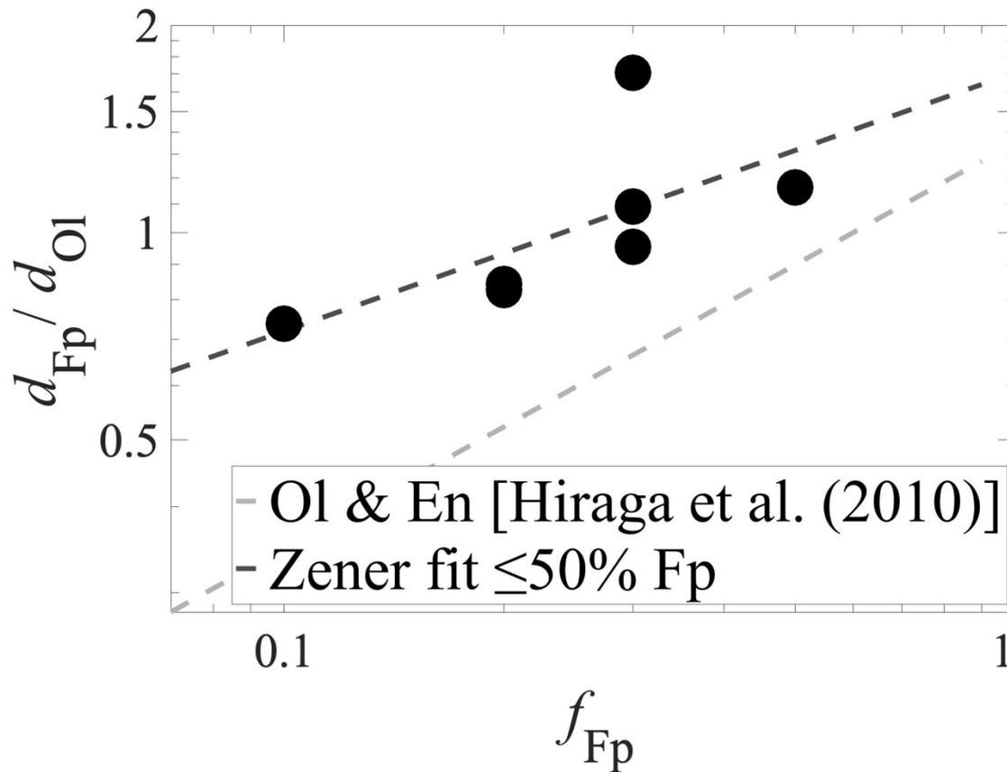
Ratio of grain sizes versus fraction of Fp for samples containing  $\leq 50\%$  Fp fit using the Zener relation. This fit yields  $m = 0.38$  indicating secondary phase particles occur predominately at three- and four-grain junctions [Evans et al. (2001)].
