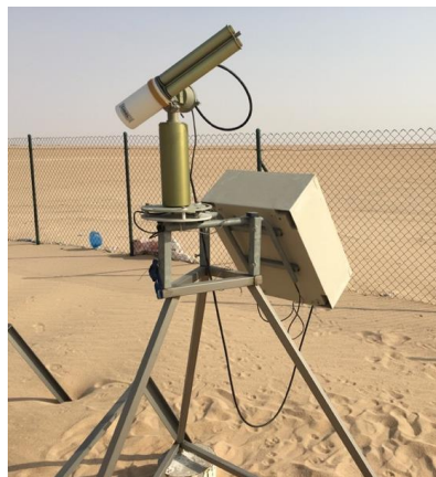
273 Figure 1. AERONET sun photometer at Shagaya Renewable Energy Park in western Kuwait. 274 Photo © 2018 by Jared A. Lee.
