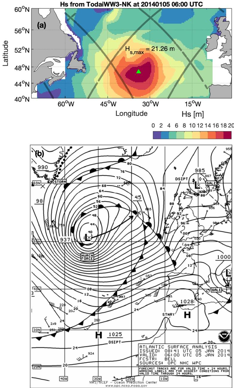
**Figure 2.** Spatial distribution of  $H_s$  from TodaiWW3-NK during the extreme event in January 2014. In subplot (a) the snapshot of  $H_s$  is shown for January 5, 2014 at 0600 UTC. The location of  $H_{s,max}$  is highlighted by a green color triangle. The altimeter tracks of JASON-2 on January 5, 2014 are plotted on top of  $H_s$ . In subplot (b) NOAA OPC synoptic analysis charts is shown for 06:00 UTC on 05 Jan 2014.
