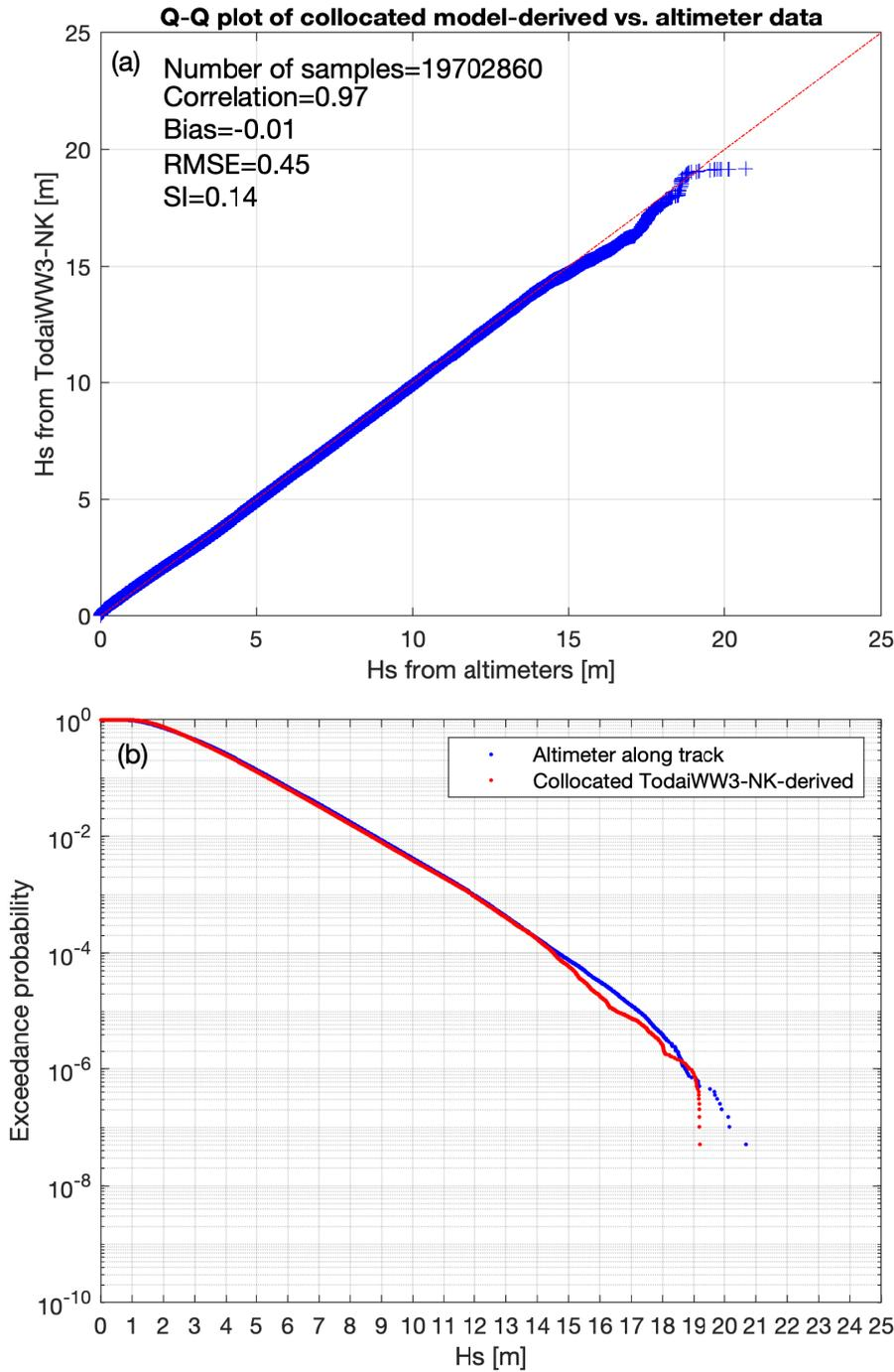
**Figure S3.** (a) Q-Q plot of Hs between TodaiWW3-NK and altimeter derived data for the GWS 8,9,15,16. (b) Comparison of exceedance probability of Hs between TodaiWW3-NK and altimeter derived data. Here the collocated model derived and altimeter along track derived data for 25 years from 1994-2018 are used for the comparison.
