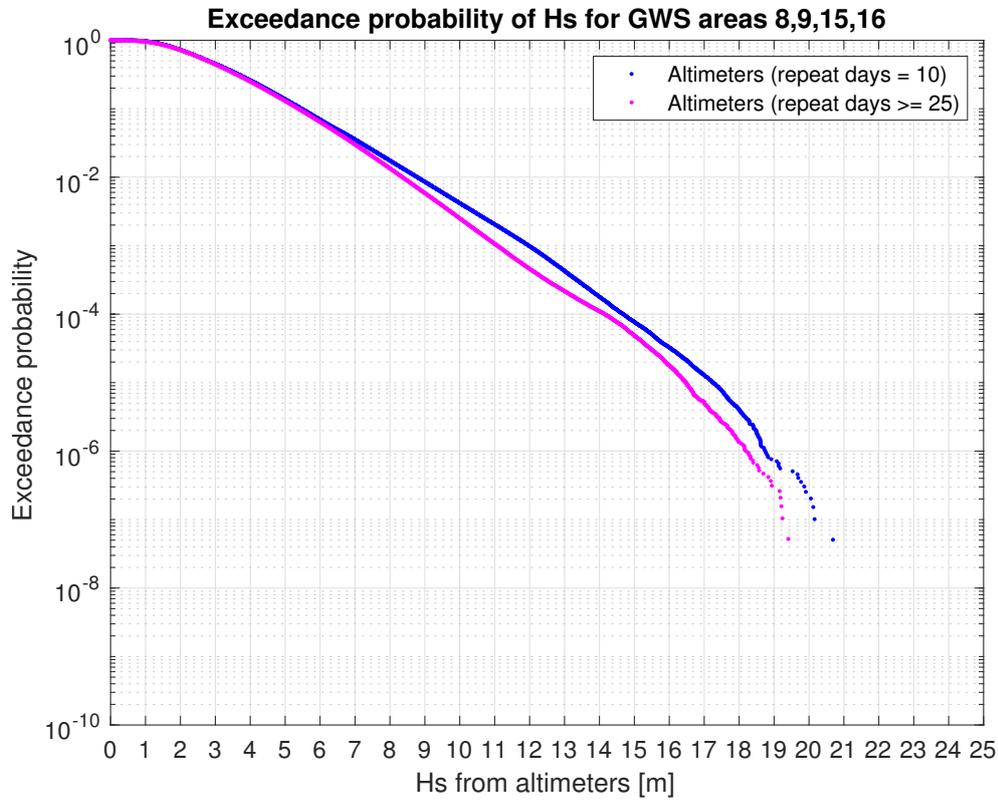
**Figure S2.** Comparison of exceedance probability of significant wave height between altimeters with repeat cycle=10 days and repeat cycle  $\geq$ 25 days. The altimeters with repeat cycle=10 days are TOPEX, JASON-1, JASON-2, and JASON-3. The altimeters with repeat cycle  $\geq$ 25 days are ERS-2, ENVISAT, CRYOSAT-2, SARAL, and SENTINEL-3A. The comparison is made for GWS areas 8,9,15 and 16 using 25 years data from 1994 to 2018.
