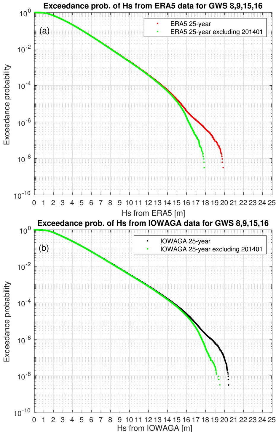
**Figure S6.** The exceedance probability of Hs is compared with and without January 2014 data. (a) Exceedance probability of significant wave height from ERA5 using 25 year 3-hourly data from 1994 to 2018 for GWS areas 8,9,15 and 16. (b) Exceedance probability of significant wave height from IOWAGA using 25 year 3-hourly data from 1994 to 2018 for GWS areas 8,9,15 and 16.
