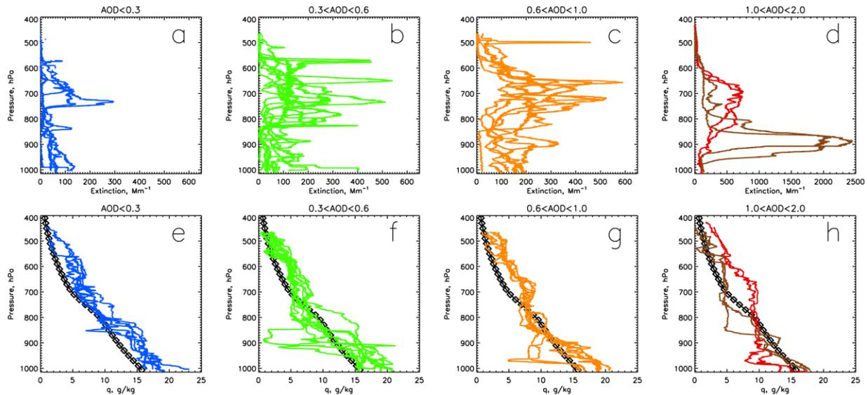
248 **Figure 2.** Aircraft profile observations of aerosol extinction (top row) and water vapor mixing
