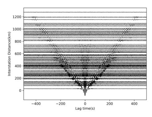
128 Fig. 2. The correlation of one-year data from the SCZJG seismic station
