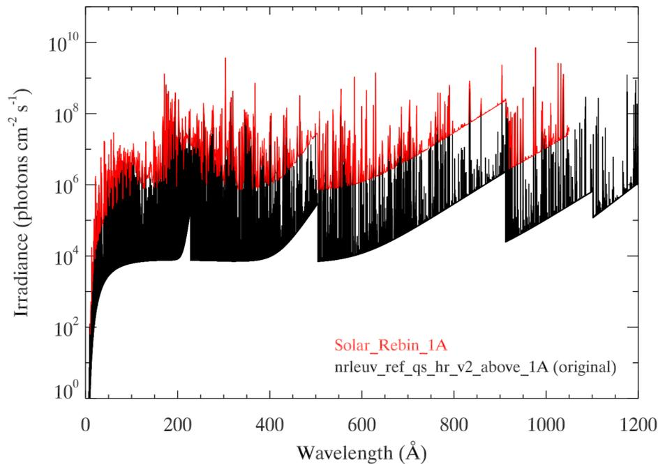
**Figure 1:** Comparison of high-resolution (0.01 Å) NRLEUV solar irradiance provided by H. Warren (black) and the same spectrum re-binned onto the low-resolution grid (red) with bin size of 0.5 Å below 100 Å and 1 Å from 100 to 1050 Å.
