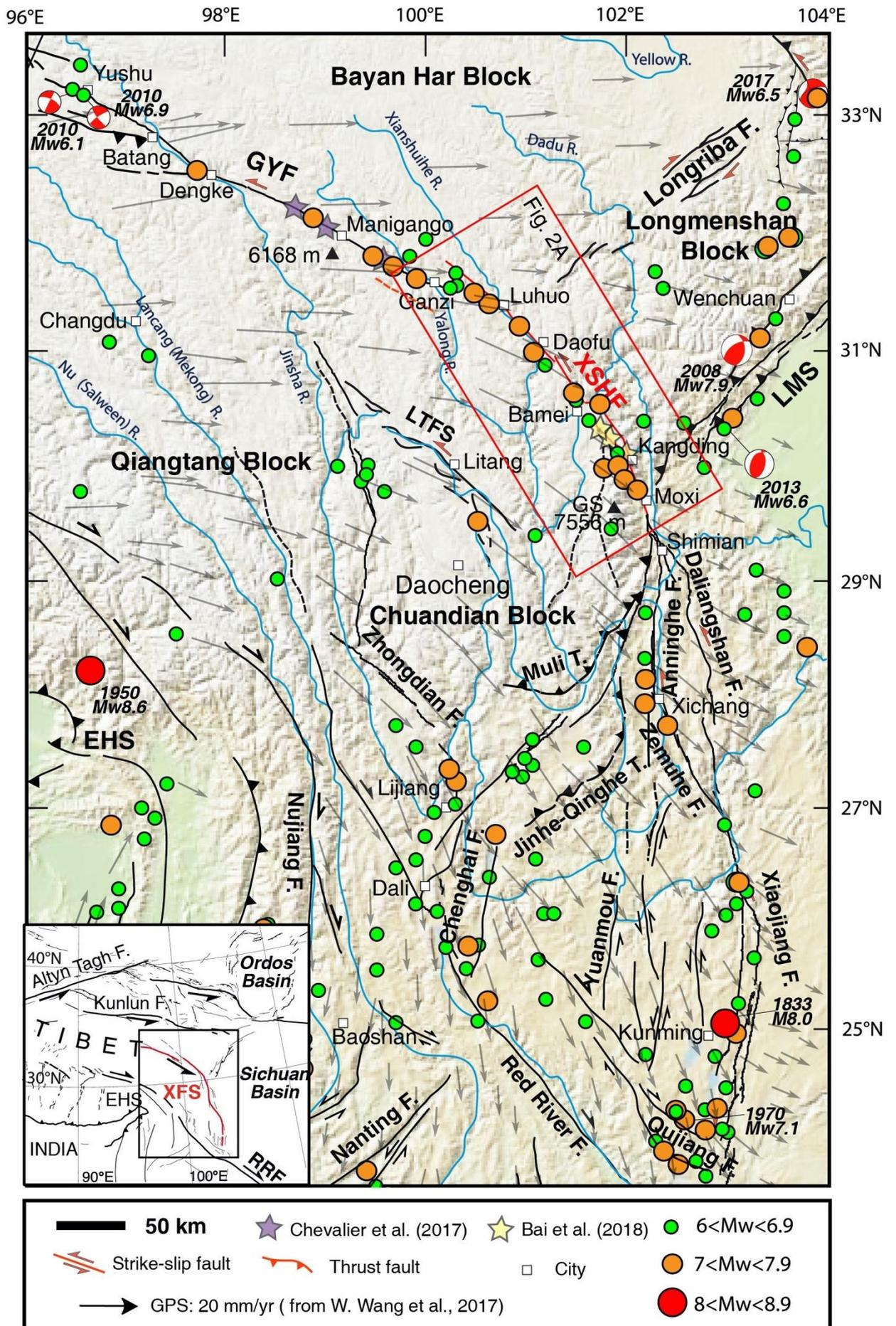
84 **Figure 1:** The Xianshuihe fault system (XFS) in the frame of the India–Asia collision zone: Tectonic
