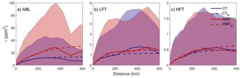
**Figure 8.** Experimental variogram for [CO<sub>2</sub>] residuals for CT and WRF at levels (a) ABL; (b) LFT; and (c) HFT. The dashed lines indicate an exponential variogram fit. Shaded areas show the standard-deviation within each bin of the experimental variogram.
