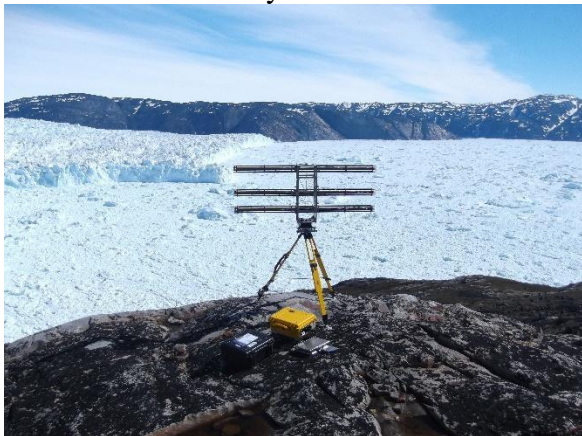
Figure 2 – Set-up of the TRI overlooking the calving front of Store.
