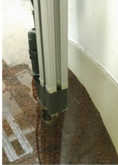
*Figure 5. Experiment pictures of (a) the dense acrylic cylinder array ( $ah=0.5$ ) with crushed walnut shells as the sediment substrate; (b) near-bed DO measurement by the optical PASCO DO sensor.*
