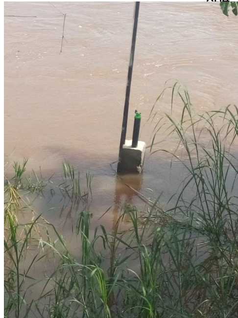
817 Figure 6 Design of a concrete housing structure of the WLL (N'sele tributary)
