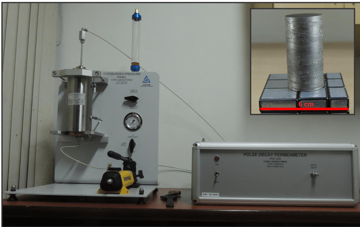
Pulse decay permeameter for gas permeability measurement. Coal cores used for measurement is in the inset.
