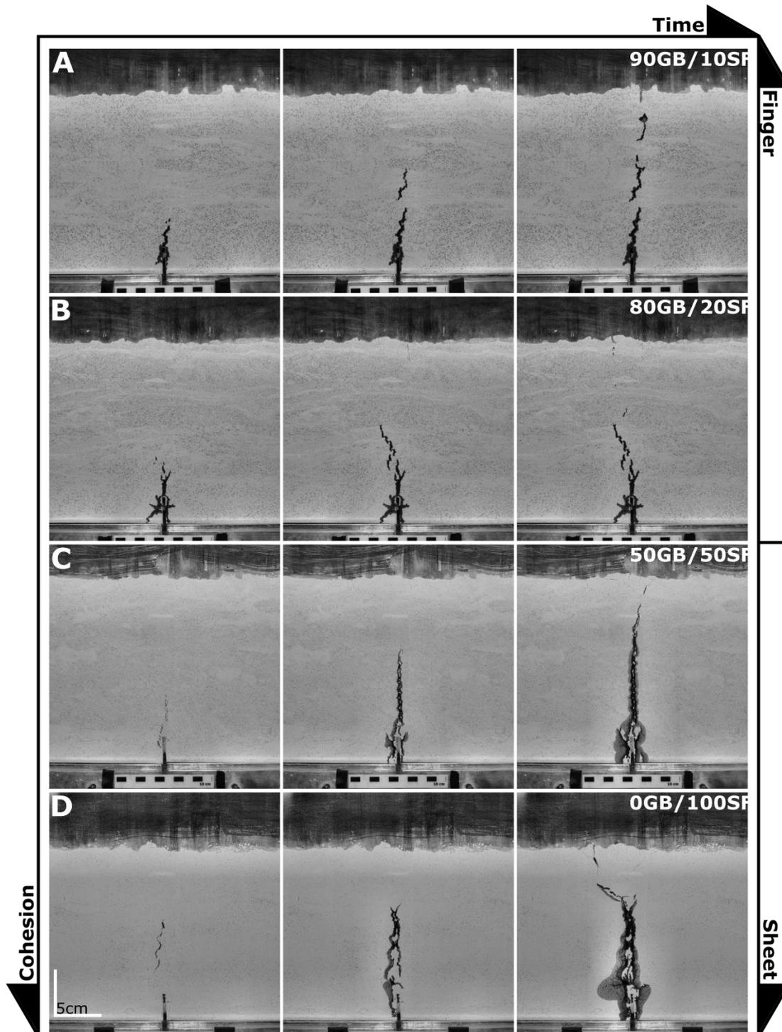
**Figure 3.** The rows show intrusion into a compacted mix of 90 wt% glass beads and 10% silica flour (A), 80/20 (B), 50/50 (C) and 0/100 (D). Columns show experiment photos at an initial, intermediate and late time step. The time steps were chosen such that they show intrusion initiation, a period of stable vertical propagation and the critical depth where failure of the overburden occurs. Experiments
