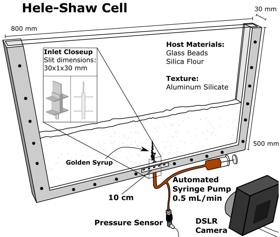
**Figure 2** Dimensions of Hele-Shaw cell including a compacted mix of cohesive silica flour and glass beads into which golden syrup is injected through the use of an automated syringe pump at 0.5 ml/min. Monitoring is done through recording of pressure and a camera taking photographs each 120/180 s depending on the mix used. We then apply digital image correlation (DIC) to the series of processed images.
