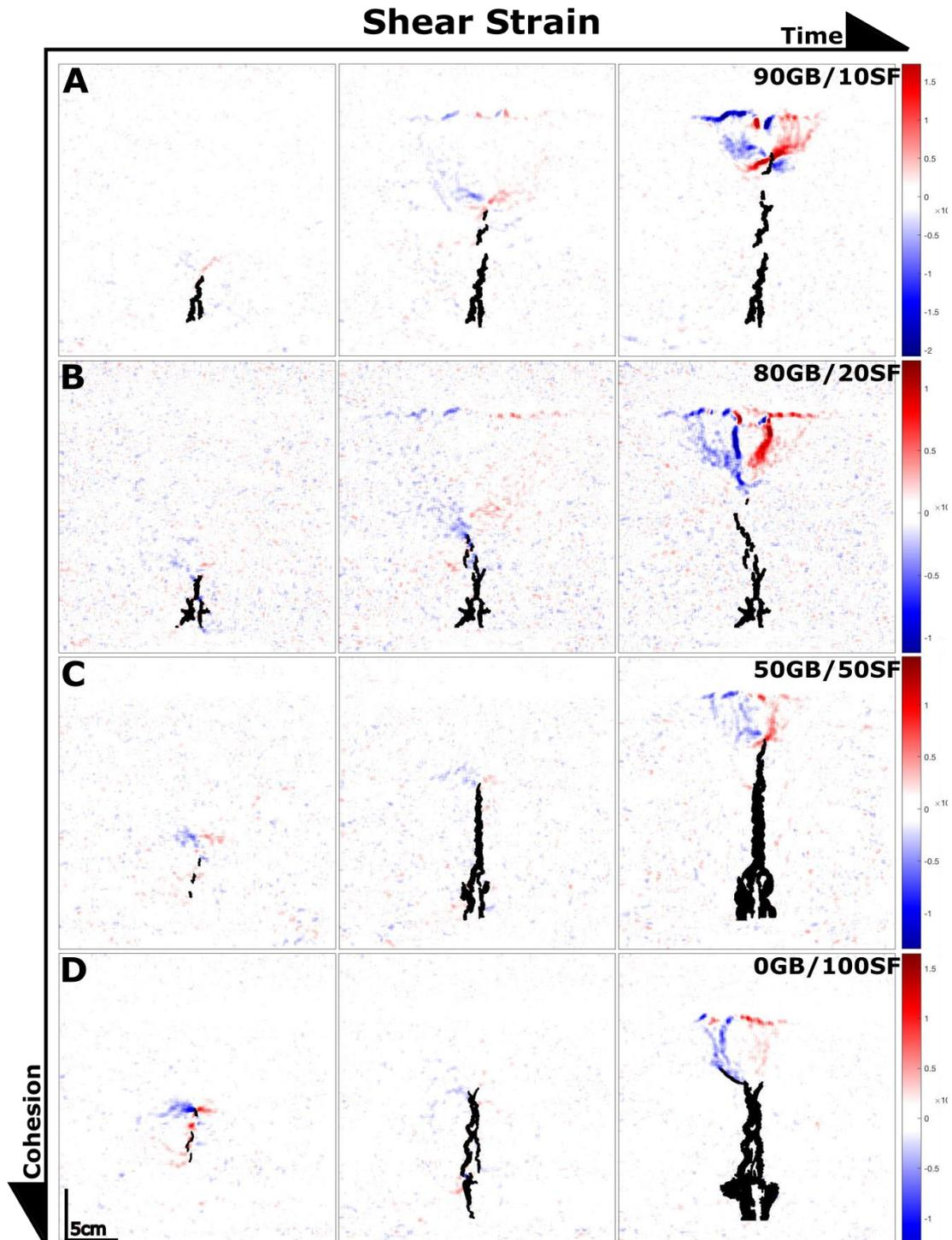
**Figure 7.** The rows show intrusions (black) into mixes of 90/10 (A), 80/20 (B), 50/50 (C) and 0/100 (D). Columns show experiment photos at an initial, intermediate and late time step. The computed shear strain in A and B extends from the intrusion already at depth until ultimately causing critical failure of the overburden. C & D shows smaller zones of shear associated with the intrusion tip. The
