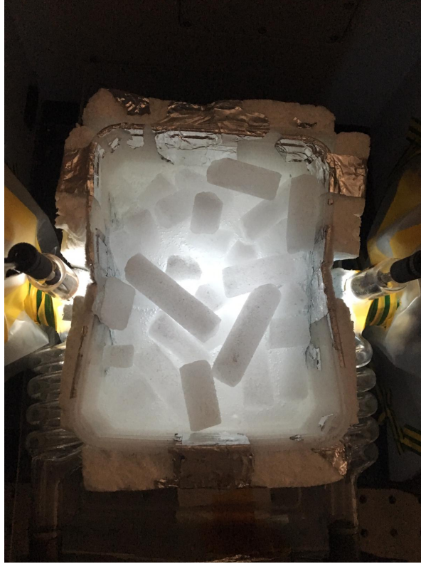
Figure 2. Discharge reactor immersed into a mixture of dry ice and ethanol and positioned in the sample compartment of the FTIR when the plasma is ON.
