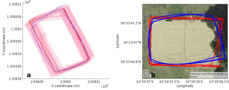
Figure 4: A rectangular volleyball field serves as ‘Proof of concept’ case. (a) Estimated rectangular path with standard deviations. Blue: The reconstruction. Red: GNSS surface drifter path. All values are given in UTM coordinates. (b) Estimation of the volleyball field with optical satellite image in the background. The reconstruction is shown in blue and the dGPS reference path in red.
