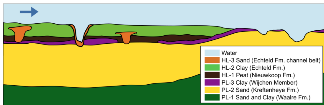
Figure 1. Conceptual longitudinal subsurface lithological longitudinal section of a river bed, with typical distances of 10 to 20 meters in depth and 10 to 20 km in length. Arrow indicates flow direction. In colour the lithological formations (Fm.) and members are indicated. Scour holes form in layers or patches composed of sandy material with lower erodibility compared to the surrounding resistant clay or peat layers.
