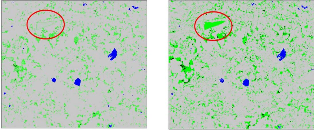
**Fig 14:** Effect of feature scaling on the segmentation of Slice 35 of Map-2. Images on left and right are segmented using Random Forest classifiers trained on unscaled features and features scaled using MinMax Scaler, respectively.
