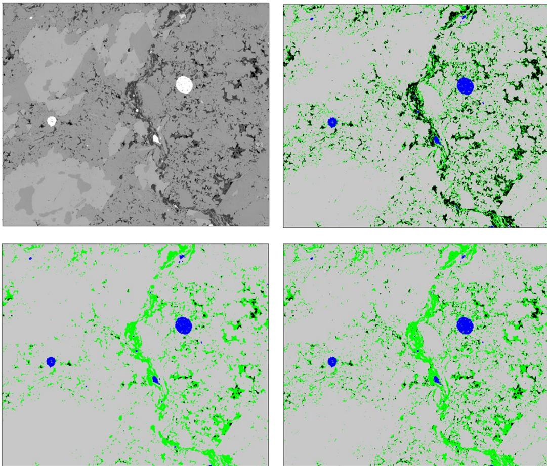
**Fig. 10:** Slice 55 from the Barnett shale (top left), after segmentation using Model-1 trained only on Wolfcamp (top right), Model-2 trained only on Barnett (bottom left) and Model-3 trained on both Wolfcamp and Barnett (bottom right).
