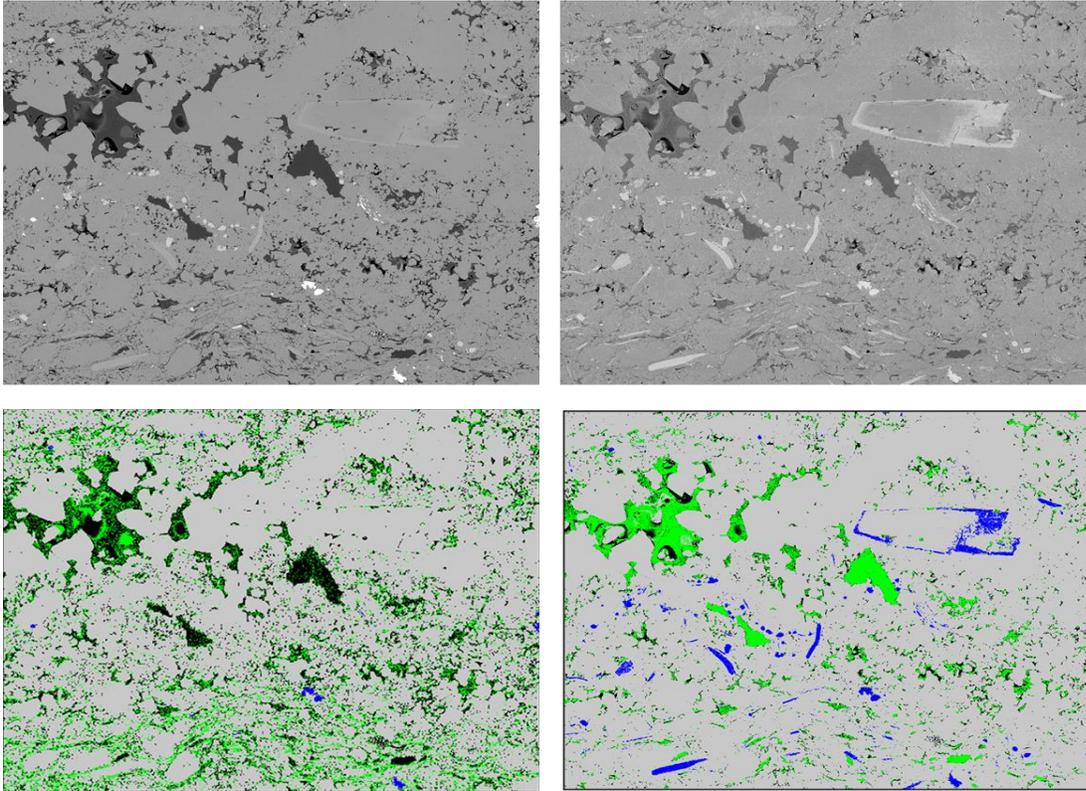
**Fig 15:** Effect of histogram equalization on Slice 28 of Map-2. Original image (top left), image after matched with histogram of Slice 90 of Map-1 (top right), original image segmented by Model-1 (bottom left), and matched image segmented by Model-1 (bottom right).
