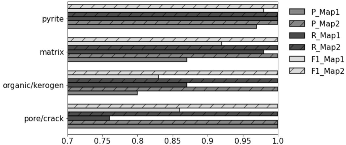
**Fig. 6:** Comparison of segmentation performance (P: precision; R: recall; F1: F1 Score) of Model-2 on inner-region test/deployment pixels of Wolfcamp against that on inner-region test pixels from Barnett. Model-2 was trained on training pixels from Barnett.
