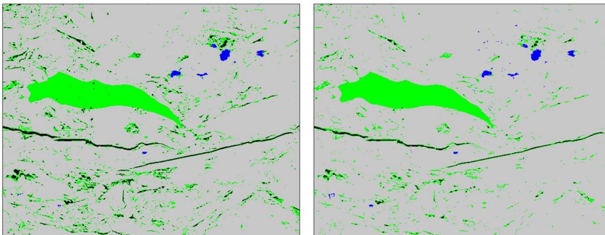
**Fig. 7:** Images showing the difference in segmentation of Slice 334 from Wolfcamp shale using Model-1 (left) and Model-2 (right). The difference is most prominent in pore/crack and organic/kerogen components.
