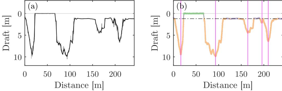
Figure 4: Example of ice draft from burst measurements: (a) Raw (thin grey line) and smoothed (black line) ice draft during a single burst ( $\sim 17$  min) in April 2019 at SODA-A. (b) The burst from (a) classified to show leads (green line), level ice (purple), and ridged ice (orange), with vertical magenta lines showing unique keels (based on Rayleigh criterion), and black dashed-dotted line showing the level ice draft classified for that burst.
