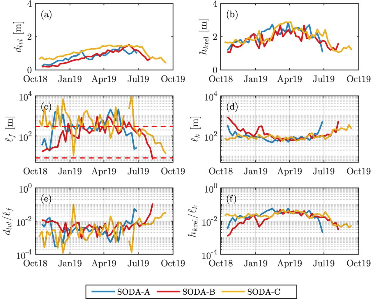
Figure 5: Weekly statistics of sea ice geometry for each mooring: (a) mean level ice draft; (b) mean relative keel height; (c) mean floe length; (d) mean keel spacing (e) aspect ratio ( $d_{lvl}/\ell_f$ ); and (f) ridging intensity ( $h_{k,rel}/\ell_k$ ). Horizontal dashed red lines in (c) show the maximum and minimum extents of the parametrized floe length (eq. 13).
