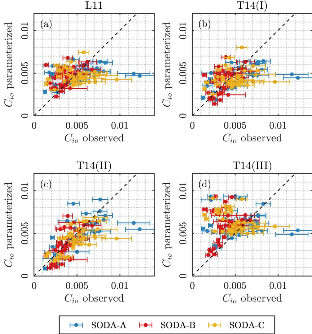
Figure 7: A comparison between the ice-ocean drag coefficients determined using the force-balance approach (“observed”), and using the different variations of geometry-based parameterization: (a) L11, (b) T14(I), (c) T14(II), and (d) T14(III). In each panel, the black dashed line shows the one-to-one slope, and the points are coloured by mooring according the legend.
