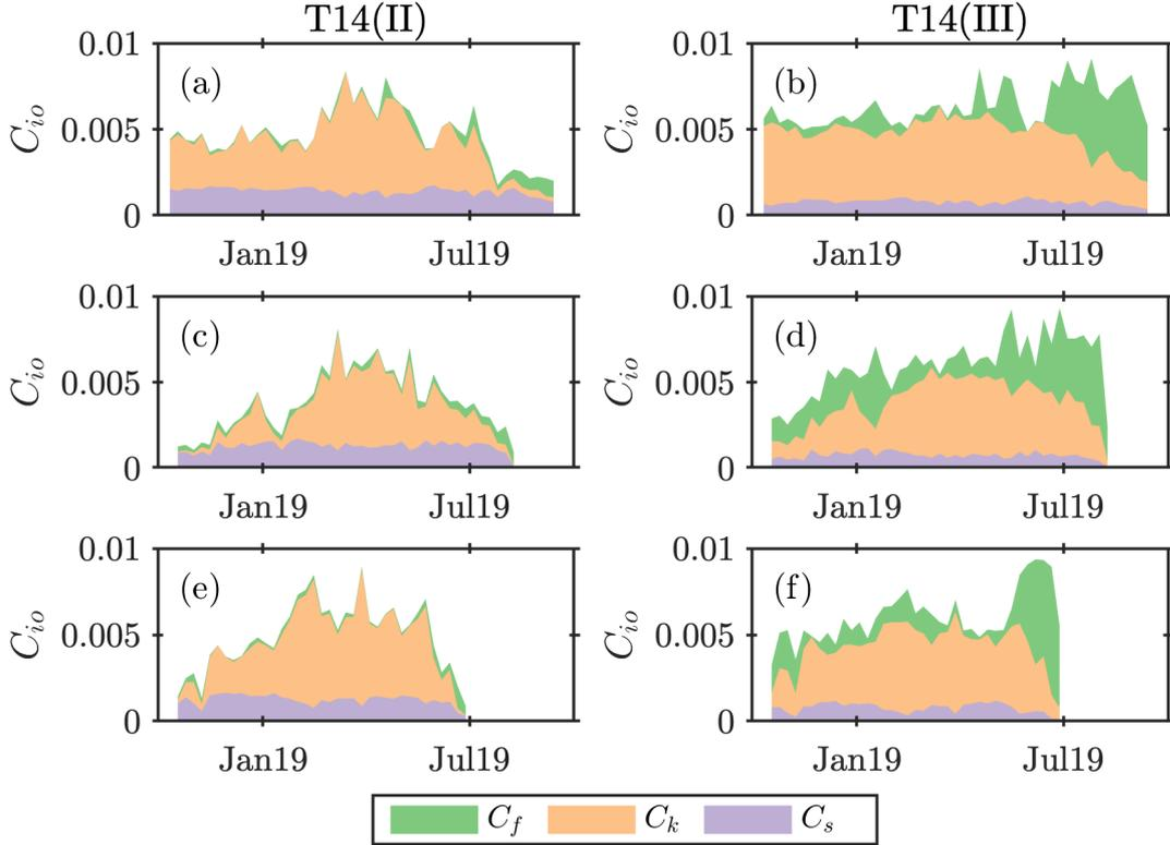
Figure 8: Stacked contributions to the ice-ocean drag coefficient  $C_{io}$  from form drag on floe edges ( $C_f$ ), form drag on keels ( $C_k$ ), and skin drag ( $C_s$ ) calculated using (a-c) the T14(II) scheme, and (d-f) the T14(III) scheme (see table 2) for (a,d) SODA-C, (b,e) SODA-B, and (c,f) SODA-A.
