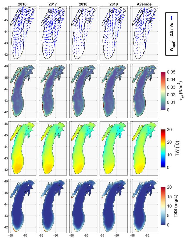
718Figure 13. Average annual wind fields ( $W_{spd}$ ), current-wave driven bottom shear stress ( $\tau_{sf}$ ), surface temperature719fields (TW), and depth-averaged total suspended solids (TSS) in Lake Michigan during the period of 2016-2019720years. The last column shows the average for four simulated years.
