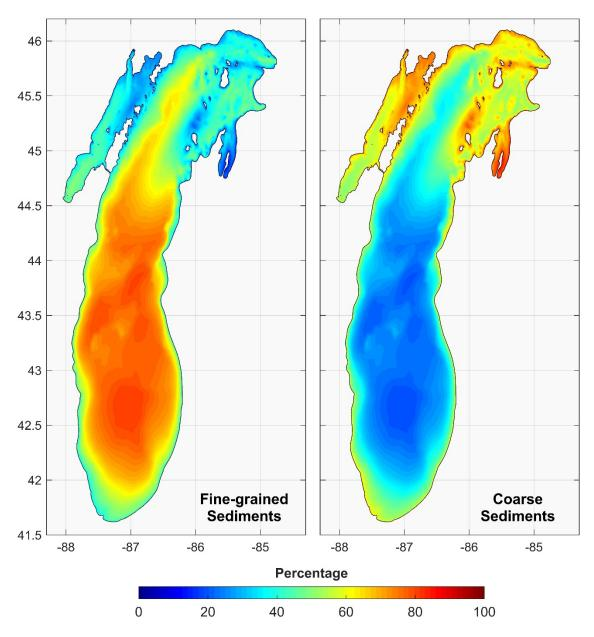
**Figure S4.** Distribution of fine-grained and coarse sediment classes in Lake Michigan used to initialize the sediment transport model. We defined Clay, Fine Silt, Coarse Silt, and Fine Sand as fine sediments and Coarse Sand, and Gravel as coarse sediments.
