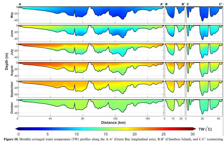
642 straits) cross-sections (as shown in Figure 1) during the period of 2016-2019 years. The vertical axis is exaggerated ~700 times.
