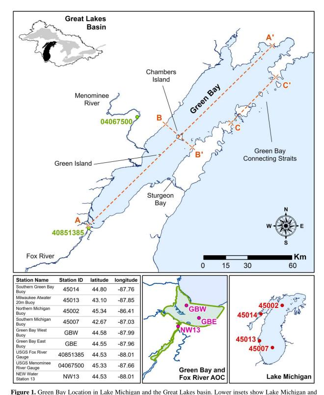
255 Figure 1. Green Bay Location in Lake Michigan and the Great Lakes basin. Lower insets show Lake Michigan and 256 Green Bay Area of Concern (AOC). Buoy stations and USGS gauges used in this study and their abbreviations are 257 also shown in the Figure. Cross-sections A-A', B-B', and C-C' are used to look at transport patterns in different
