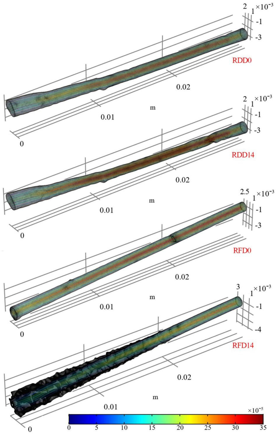
**Fig. 4** Demonstration of 3D fractures and velocity streamline.
