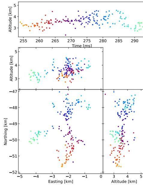
**Figure 6.** Floating threshold windowing with the LMA-emulator, centered on a negative leader in the 2018 flash. Showing 173 sources that have 8 or more participating stations.
