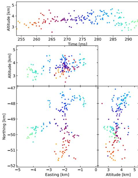
**Figure 5.** Non-aligned windowing with the LMA-emulator, centered on a negative leader in the 2018 flash. Showing 164 sources that have 8 or more participating stations.
