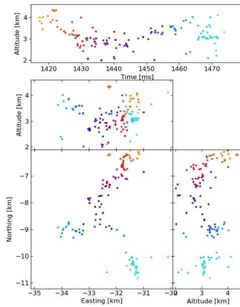
**Figure 10.** Floating threshold windowing with the LMA-emulator, centered on a negative leader in the 2019 flash. Showing 130 sources that have 8 or more participating stations.
