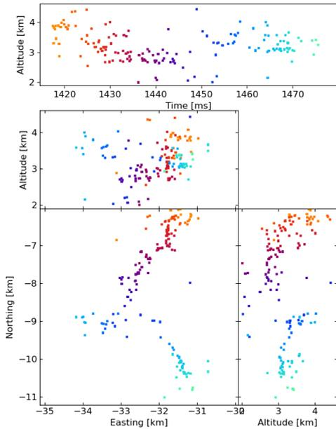
**Figure 9.** Non-aligned windowing with the LMA-emulator, centered on a negative leader in the 2019 flash. Showing 154 sources that have 8 or more participating stations.
