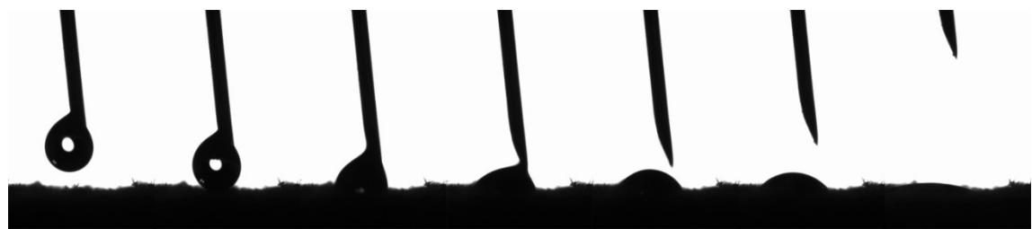
Fig. 2. Process of the contact angle measurement between the aqueous ethylene glycol solution and black soil at -10°C.
