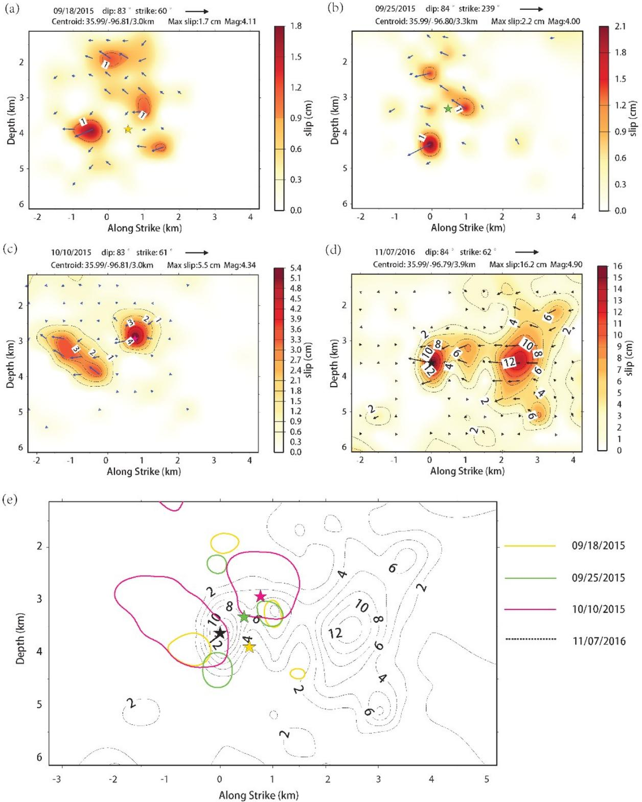
590Figure 5. Rupture models from finite fault inversion of (a) the 09/18/2015  $M_w$  4.1, (b) the
