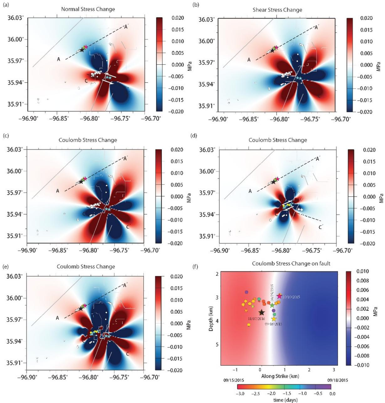
637Figure 9. Coulomb stress changes resolved on right-lateral fault, striking 60 degrees with
