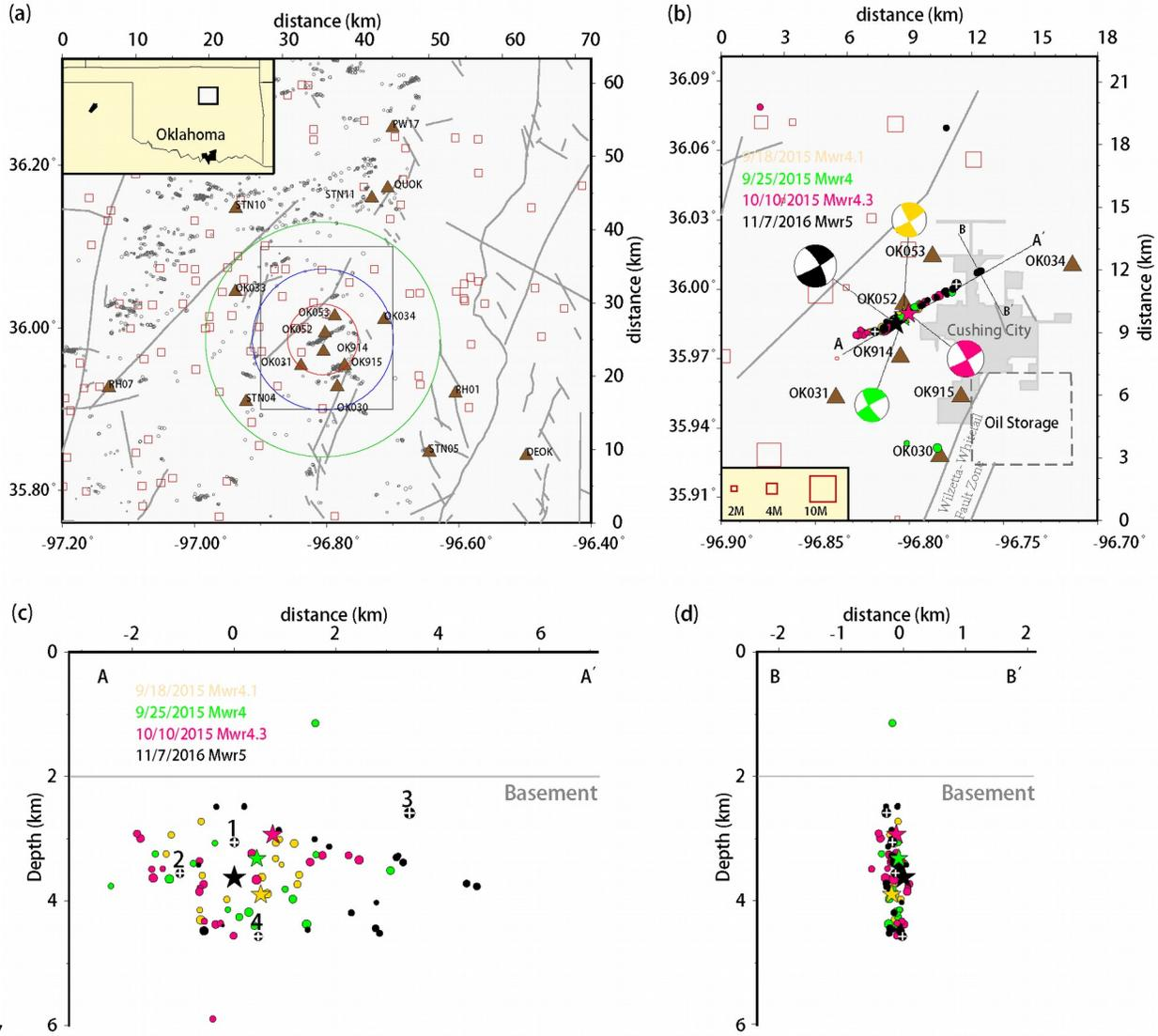
548 Figure 1. Seismicity near Cushing city, and seismic stations and disposal wells. (a) Seismicity
