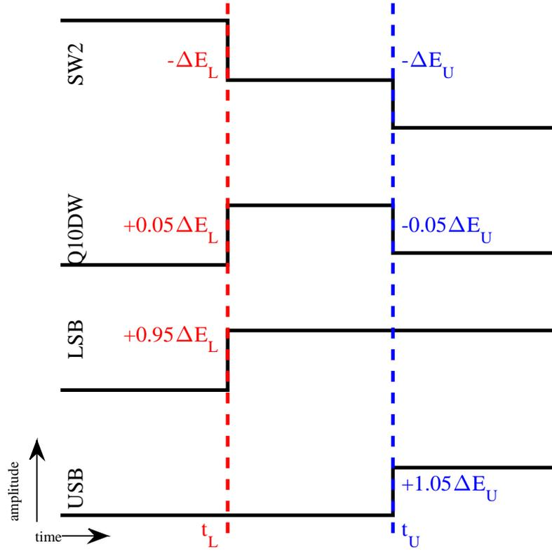
Figure 4: A sketch of net energy gain of the four waves in the Q10DW-SW2 nonlinear interactions according to the Manley-Rowe relation. The red and blue represent the LSB- and USB-generating interactions occurring at  $t_L$  and  $t_U$ , respectively. Between  $t_L$  and  $t_U$  maximizes the Q10DW.  $\Delta E_L$  and  $\Delta E_U$  are energy exchanged through SW2.
