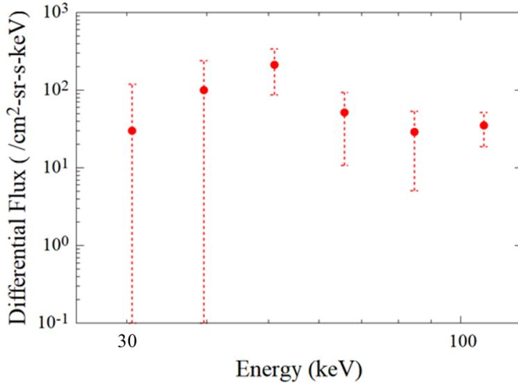
231 Figure 6. Calibrated energy spectrum of precipitating electrons. Error bars indicate  $2\sigma$ , where
