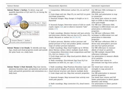
Figure 1. ASPEN instrument science themes, measurement objective and instrument requirements [1].
