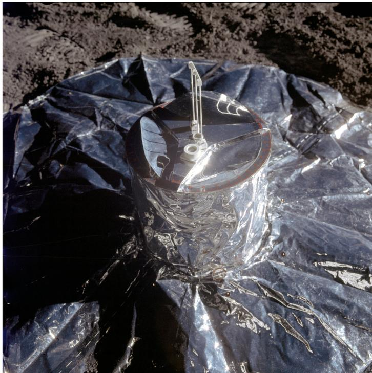
Figure 9: Gnomon used on the Moon with the passive seismic experiment (PSE) during the Apollo 14 mission.
