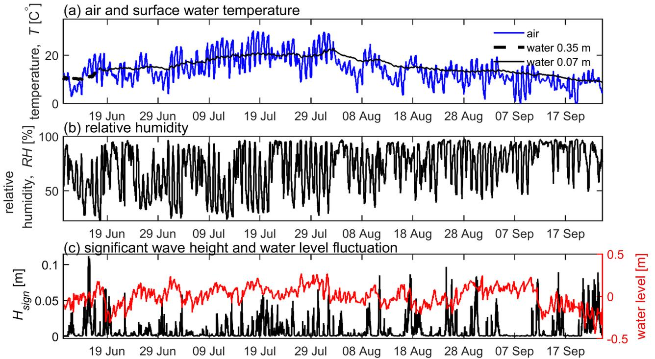
**Figure S4.** Time series of (a) air temperature (at 2 m height above the water, blue line) and surface water temperature (at 0.35 and 0.07 m depth, black line); (b) relative humidity. Significant wave height  $H_{sig}$  (black line) and water level fluctuations (red line). All data are shown as 10 min averages.
