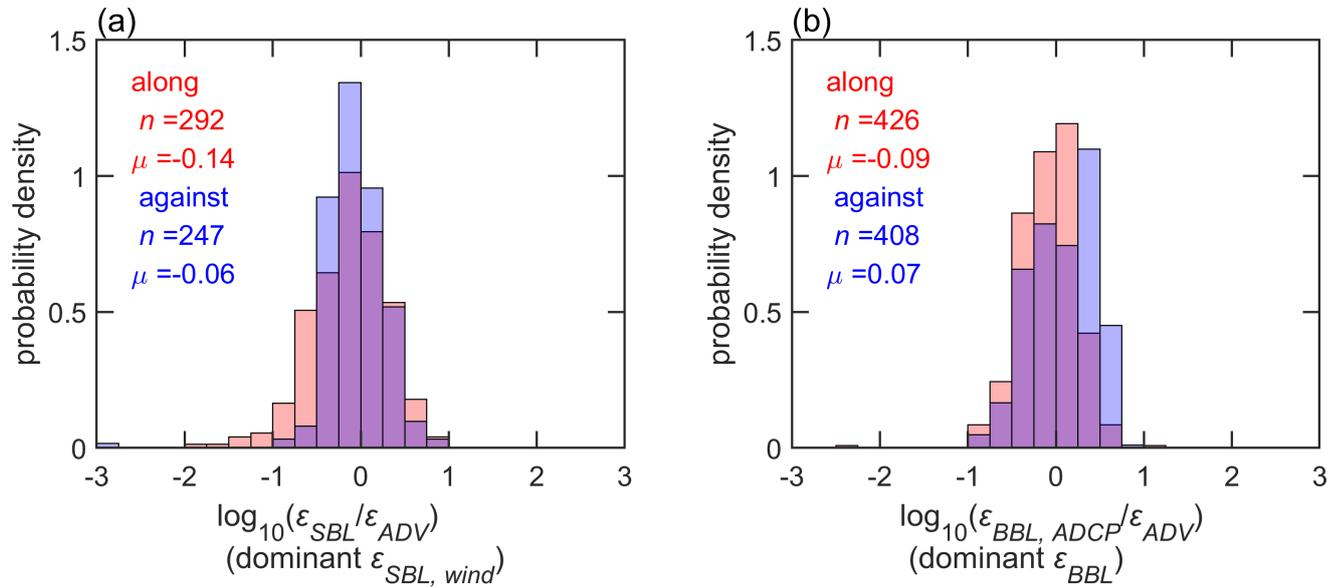
**Figure S11.** Probability density distributions of the ratio of predicted and observed dissipation rates for cases when wind was along the river flow ( $290^\circ \leq w_{dir} \leq 323^\circ$ , red) or against the flow ( $151^\circ \leq w_{dir} \leq 190^\circ$ , blue) for the situations when: (a) wind and (b) flow was the dominant driver of the near-surface turbulence. The respective number of data points  $n$  and mean  $\mu$  value of the logarithm of the ratio are shown the legend.
