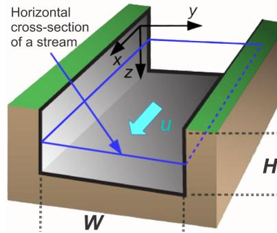
**Figure 3.** Schematic of a river channel geometry assumed in 1D  $k - \epsilon$  turbulence model
