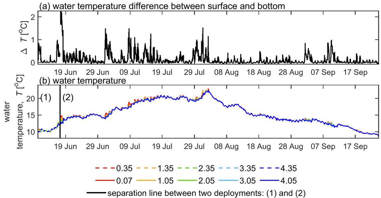
**Figure S5.** Time series of (a) water temperature difference between surface and bottom; (b) water temperature at different depths. The vertical black line separates two deployments periods of the thermistor chain: (1) 06.06 - 17.06 and (2) 17.06 - 24.09. All data are shown as 10 min averages.
