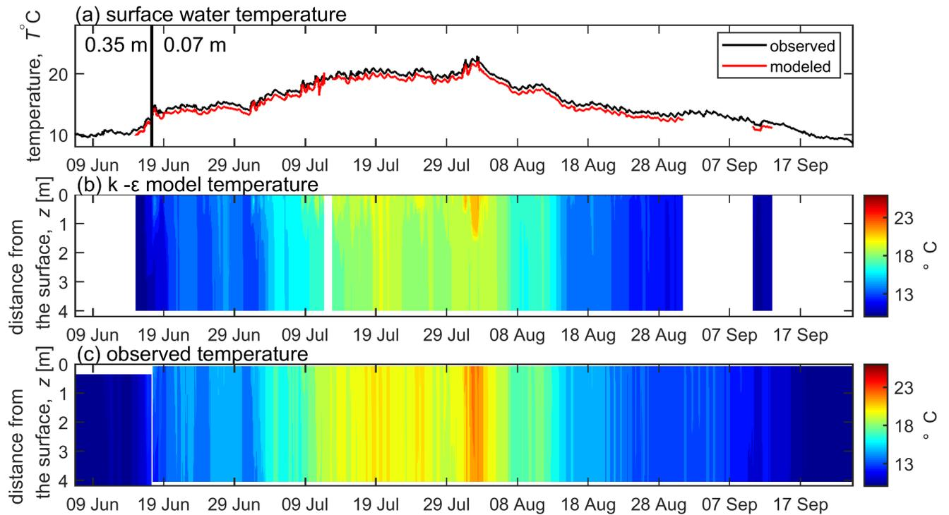
**Figure S13.** Time series of (a) surface water temperature: observed (black line) and modeled by  $k - \varepsilon$  model (red line), vertical black line separates two deployments of the thermistor chain, numbers indicate water depth (0.35 m and 0.07 m), modeled temperature was interpolated; (b) modeled water temperature profiles; (c) observed water temperature profiles.
