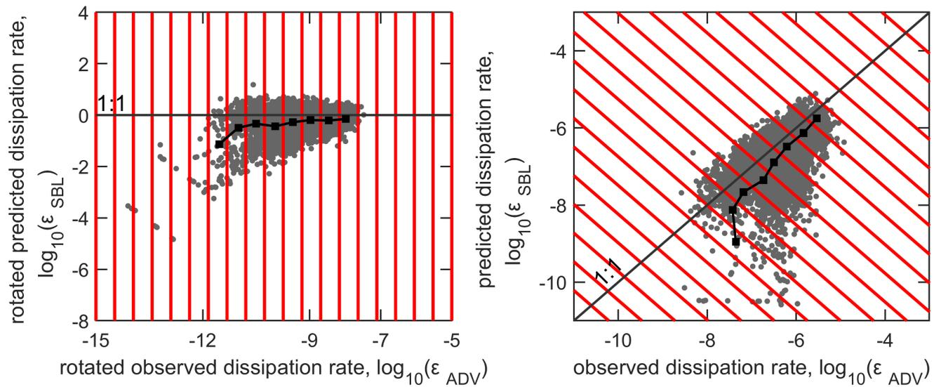
**Figure S7.** An example of logarithmic bin averaging of the data using measured  $\epsilon_{ADV}$  and predicted  $\epsilon_{SBL}$  dissipation rates from Sect. 3.2. Grey dots show: (a) rotated data ( $-45^\circ$ ); (b) original data. The solid dark grey line shows a 1:1 relationship, red lines indicate the selected intervals for averaging. The black line with square symbols shows the logarithmic bin average of the data.
