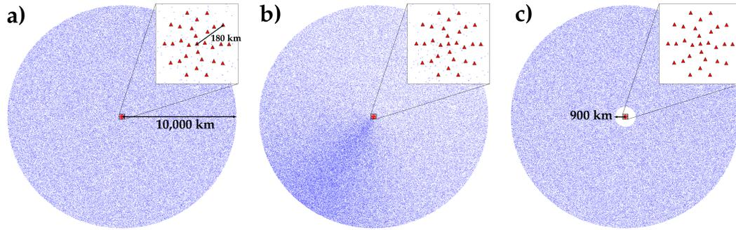
**Figure 1.** Sources (blue dots) and stations (red triangles) used for simulating seismic noise. (a), (b), and (c) indicate the source distributions used in Sections 4.1 (uniform source distribution), 4.2 (azimuth-dependent source density), and 4.3 (no sources in the near field), respectively.
