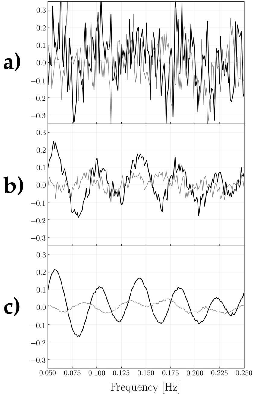
**Figure 6.** Same as Fig. 2, but obtained through the experimental setup of Section 4.2 (azimuth-dependent source density). Inter-station distance is 67,600 m. Real (black) and imaginary (gray) parts of the cross correlation obtained from the ensemble-average over 25, 500, and 25,000 realizations are shown in subpanel (a), (b), and (c), respectively.
