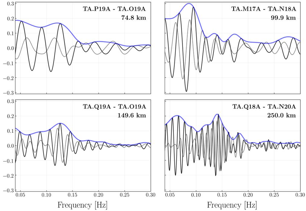
**Figure 12.** Envelopes (blue), real (black), and imaginary part (gray) of the normalized cross correlations calculated for 4 different pairs of receivers. Within each subplot, station codes and inter-station distance are indicated on the upper right.
