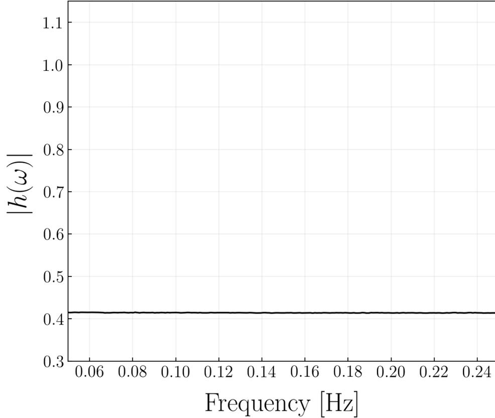
**Figure 9.** Same as Figs. 3 and 7, but obtained through the experimental setup of Section 4.3 (no sources in the near field). The absolute value of source amplitude  $|h(\omega)|$  has been retrieved from synthetic data by taking the square root of the RHS of eq. (6). Note that noise has been simulated using a constant  $h(\omega) = 1$ .
