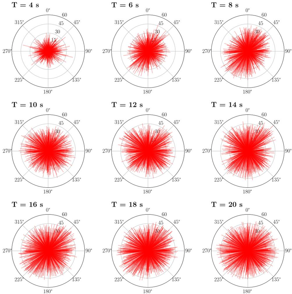
**Figure 13.** Signal-to-noise ratio at different periods as a function of azimuth, as inferred from the normalized cross-correlations. The length of the red segments is determined by the value of SNR, while their orientation coincides with the azimuth/back-azimuth of the respective station pair.  $0^\circ$  corresponds to the north,  $90^\circ$  to the east, etc.
