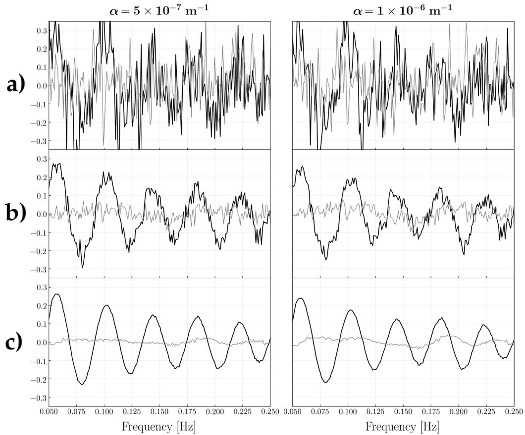
**Figure 2.** Real (black) and imaginary (gray) parts of LHS of eq. (10), obtained for a pair of receivers with inter-station distance of 67,600 m by ensemble-averaging over (a) 25, (b) 500, and (c) 25,000 realizations. Results are shown for both values of  $\alpha$  used in the experimental setup of Section 4.1 (uniform source distribution).
