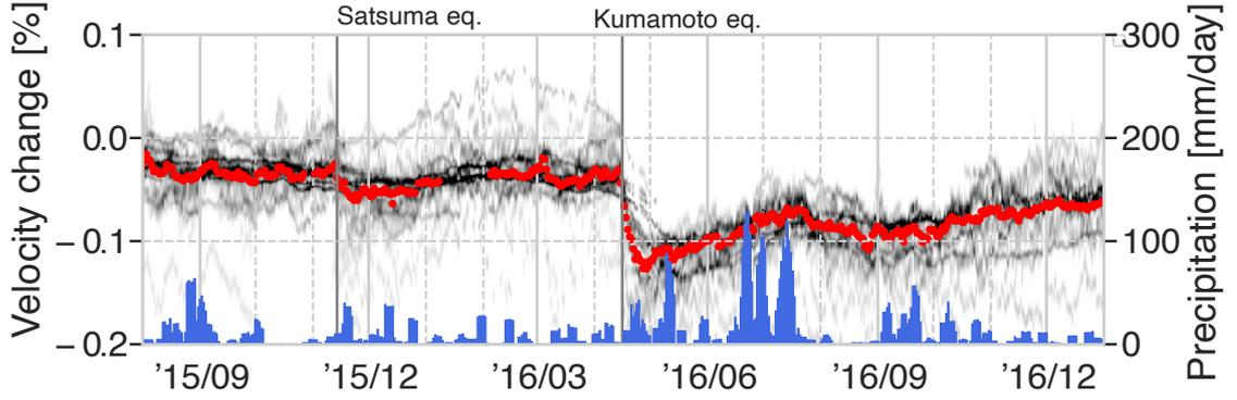
**Figure 6.** Velocity change associated with the 2016 Kumamoto earthquake. The seismic velocity drop when the earthquake occurred, and recovered over a time scale of three months. The grayscale shows marginal probability with all CCFs (see next section for details). The red dots show a median of all the measurements. The red dots also show a minor drop during the 2015 Satsuma earthquake.
