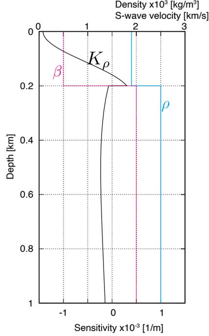
**Figure 5.** Depth sensitivity kernel to density perturbations at 0.6 Hz. The density  $\rho$  and the S-wave velocity  $\beta$  are plotted. P-wave velocities are 1.91 km/s from 0 to 0.2 km, and 4 km/s below 0.2 km.
