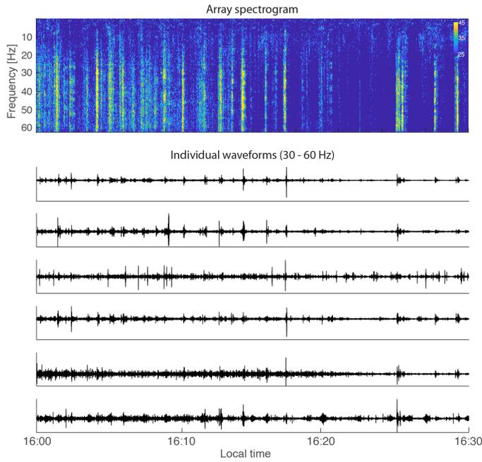
**Figure 7.** Seismic observations during a lightning storm on 11th March 2019. Top panel: array spectrogram. Bottom panels: representative waveforms at randomly selected stations around the island, filtered 30 - 60 Hz.
