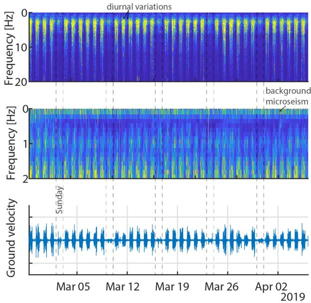
**Figure 2.** Spectrogram for frequencies less than 20 Hz (top row) and frequencies less than 2 Hz (middle row), plus the waveform (bottom row) for a node deployed in a park, after removing the instrument response.
