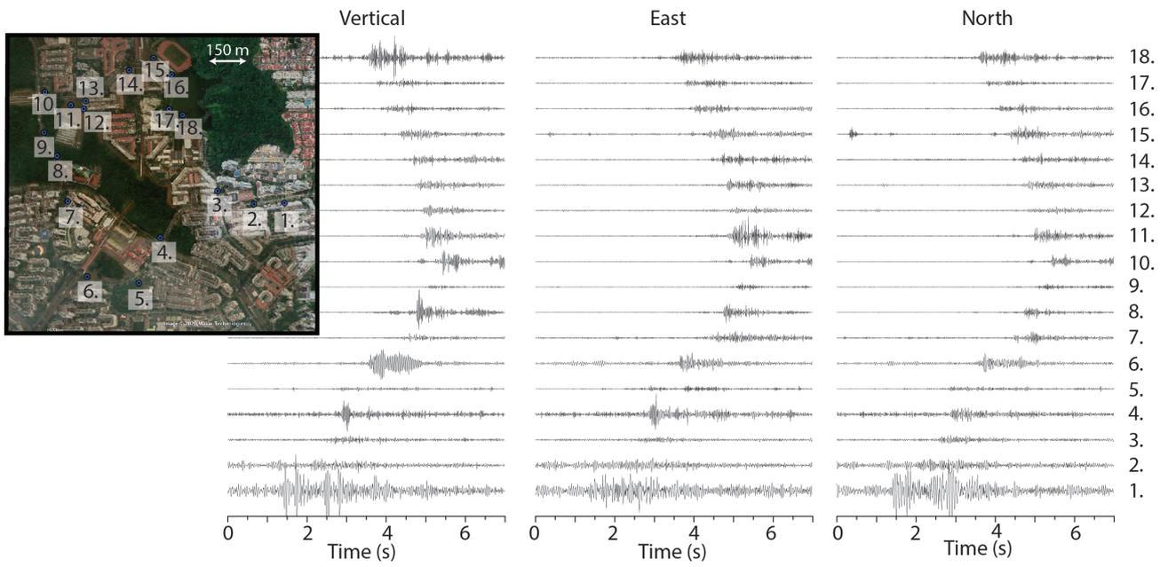
**Figure S3.** Waveforms induced by thunder at 18 stations within a 1 km x 1 km area. Waveforms are highly variable across the area likely affected by nearby buildings and near-surface structures.
