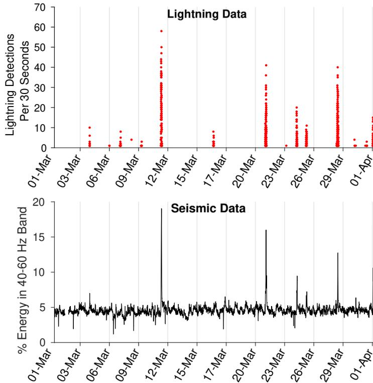
**Figure 8.** Correlation between high frequency seismic energy and frequency of lightning detected in Singapore. Seismic energy is calculated as the ratio of the average energy in the 40-60 Hz to the total seismic energy less than 60 Hz averaged for the whole array. Lightning strikes are cloud to ground lightning detected by Singapore’s lightning detection system.
