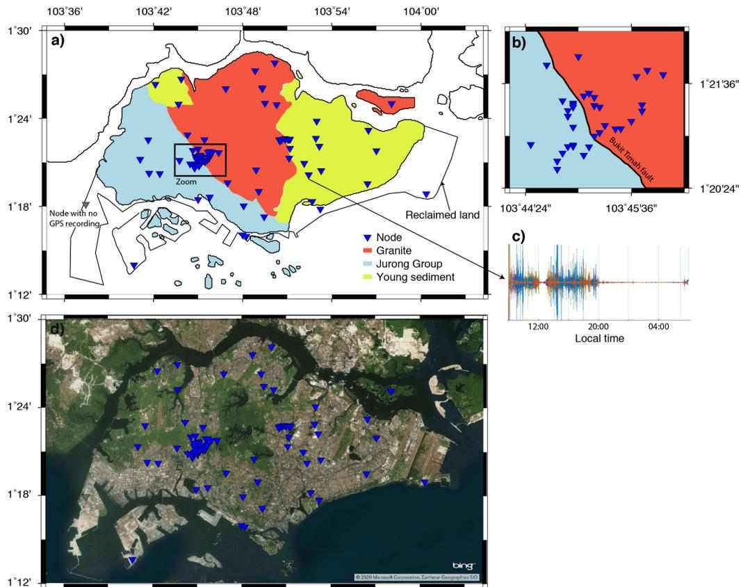
**Figure 1.** a) A simplified geological map of Singapore showing locations of nodes as blue triangles. White land areas within the Singapore coastline are reclaimed lands. b) Zoom to area of dense deployment across the Bukit Timah fault. c) Seismic data recorded by a node deployed in a school for a period of one day. Quiet times are during the lunch break and between 8pm and 8am. d) A satellite photo of Singapore with location of nodes as blue triangles.
