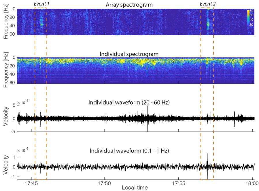
**Figure 5.** Two local events on 3rd March 2019 marked by orange boxes. Panels from top to bottom: array spectrogram; spectrogram at one station; waveform at same station filtered 20 - 60 Hz; same waveform filtered 0.1 - 1 Hz.
