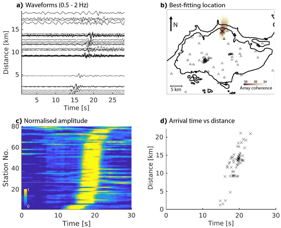
**Figure 6.** Local event on 3rd March 2019 (Event 2 in Figure 5). a) Waveforms recorded at stations in array, filtered 0.5 - 2 Hz. b) Map of Singapore with best-fitting location of source (cross) obtained by grid search of lag times. c) Moving mean of the absolute amplitude in 0.5 - 2 Hz frequency band vs stations ordered in distance from the best-fitting location. d) Move-out across the array, where distance is from the best-fitting location. Crosses mark the time of maximum amplitude from c).
