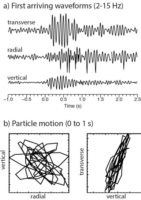
**Figure S4.** a) First arriving waveforms induced by a thunder source at red coloured station in Figure 10 (same as station number 6 in Figure S3). Horizontal components have been rotated to radial and transverse directions for the best-fitting event location. b) Particle motion for the first 1 second is consistent with a Rayleigh wave.
