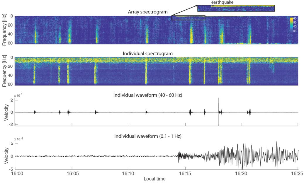
**Figure 9.** The concurrent arrival of seismic waves from an earthquake in Sumatra and a series of discrete lightning quakes. Seismic waves from the earthquake arrive at low frequencies, while the lightning quakes are across all frequencies.
