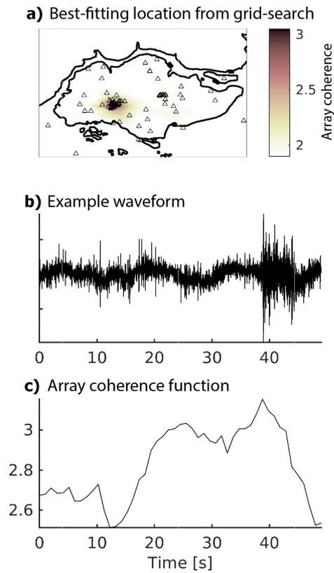
**Figure S2.** Thunder quake at around 2 am on 1st April 2019. a) Location obtained by grid search, with the best-fitting location defined as the point that maximises the array coherence. b) Example waveform (raw) c) Array coherence function.
