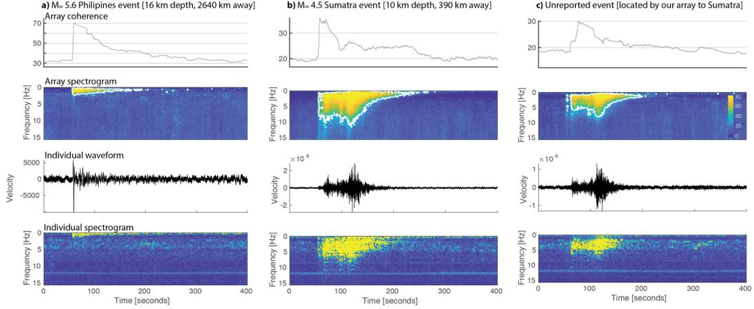
**Figure 4.** Examples of distant earthquakes detected by our array - a) an earthquake in the Philippines, b) an earthquake in Sumatra, c) an earthquake not reported in global earthquake catalogues, which we locate using the Singapore array to Sumatra. Panels from top to bottom: array coherence function; array spectrogram; waveform at one station (raw); corresponding single station spectrogram for the waveform.
