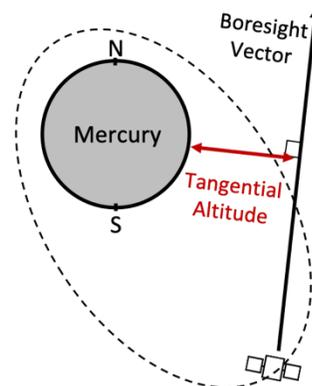
**Fig. 1.** Geometry of MESSENGER MESSENGER orbits Mercury in a long north-south orbit with high eccentricity. The shortest distance between the boresight vector and the surface of Mercury is called tangential altitude.
