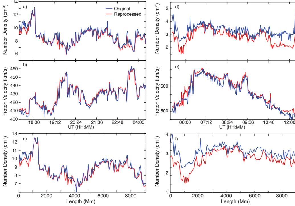
**Figure 1.** Comparison of the original (blue) and reprocessed (red) solar wind data from Wind SWE for a representative segment, for both slow (left) and fast (right). Reprocessed data show slightly lower density (a and d), slightly higher velocity (b and e), and the high frequency variations are of lower amplitude than the original data.
