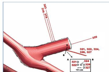
Task 9C concerns the combined predictive (earlier stage) and inverse (later stage) modelling of tracer breakthrough curves of the Through Diffusion Experiment (TDE). This in-situ tracer test has been carried out within the REPRO programme at about 400 m depth at the ONKALO underground rock characterisation facility in Olkiluoto, Finland, by Posiva.
