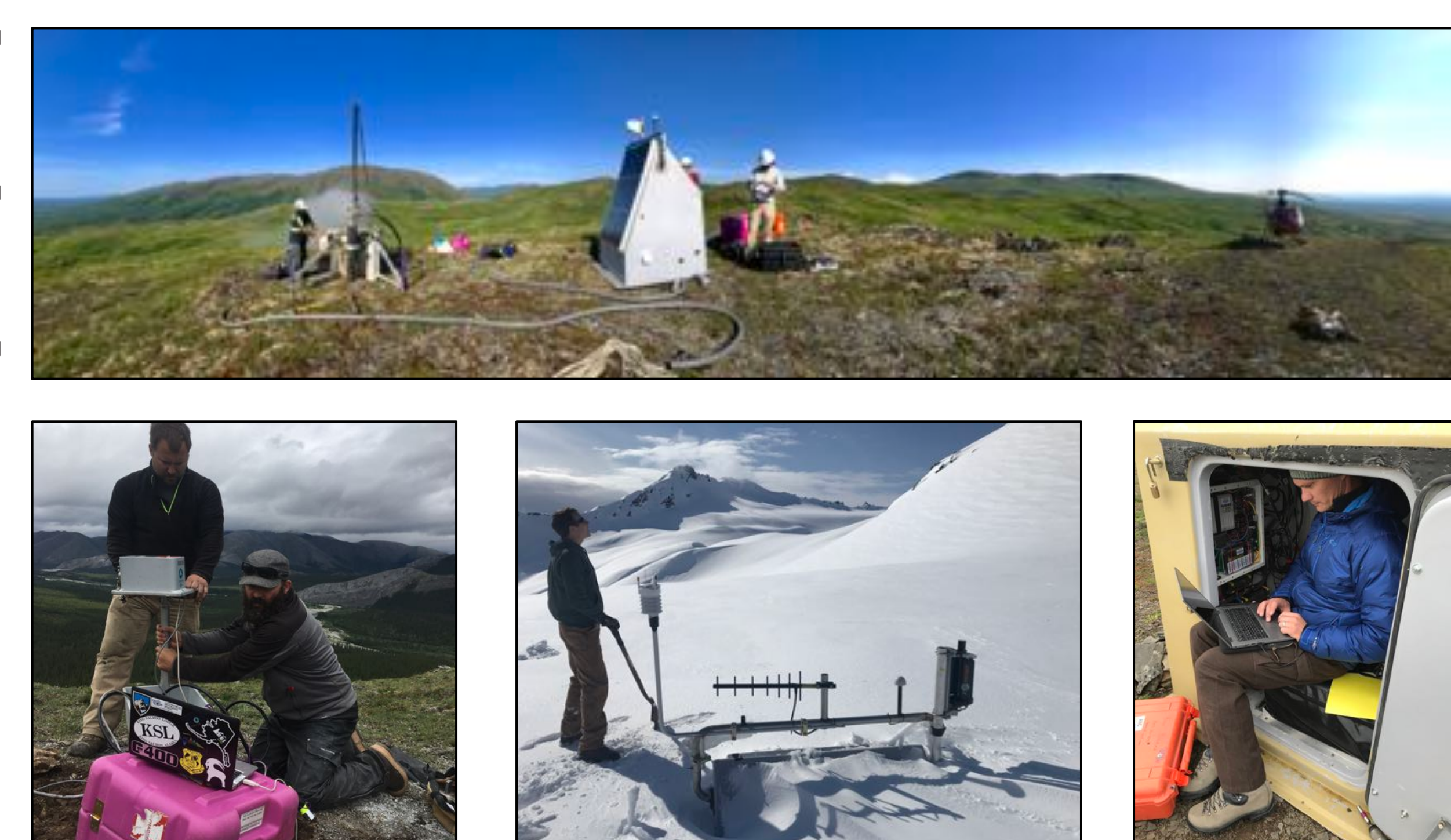
The Alaska TA (2015-2020) deployed a fixed array of posthole seismometers in remote locations using a portable drilling rig. Stations leveraged new power and communication technology to operate autonomously in harsh environments.
