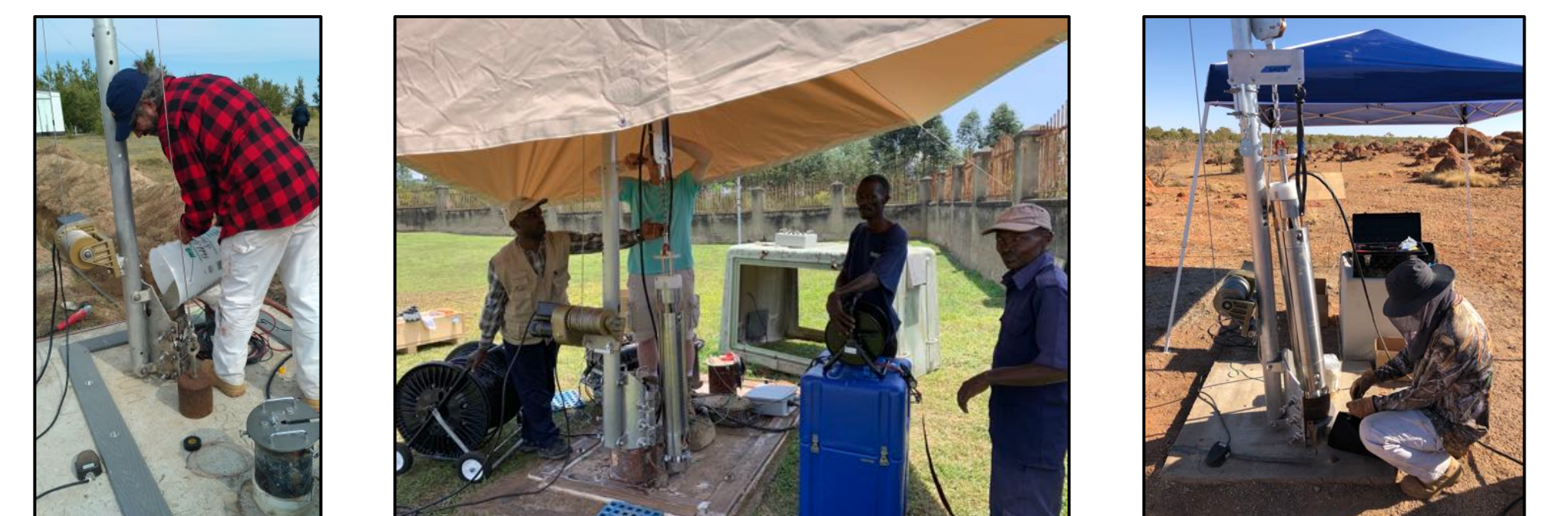
Borehole sensors at IDA network (II) stations KURK (Kazakhstan), MBAR (Uganda), and WRAB (Australia) were upgraded in 2019.
