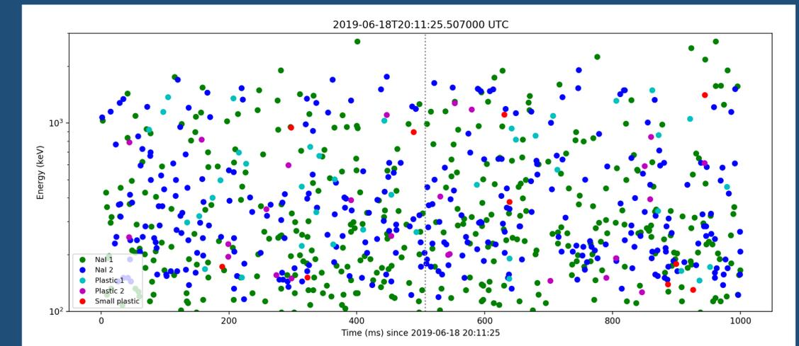
Figure 3: Scatter plot of photon energy as a function of time for events surrounding the 92 kA -CG that struck ~1.8 km away on 18 June 2019 at 20:11:25Z. Events are color-coded by scintillator. No excess events from the approaching stepped leader are visible. Attenuation of hard X-rays is expected in the intervening atmosphere and materials of the building in which the detectors are housed.
