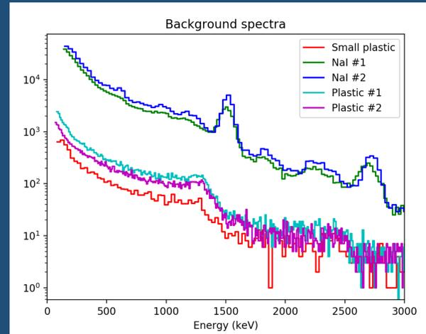
Figure 2: Sample background spectrum in each of the five scintillators. Prominent background lines are visible in the NaI(Tl) detectors at 1460 keV from <sup>40</sup>K and 2614 keV from decay of <sup>232</sup>Th. Compton back-scatter peaks from the two lines are visible in the plastic scintillators.
