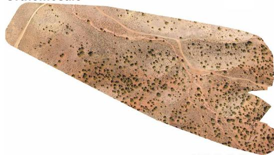
Left: This simple orthomosaic and DEM from Parowan Gap, UT was created using a DJI Phantom 3 Professional illustrating what can be done with a commercial system.
