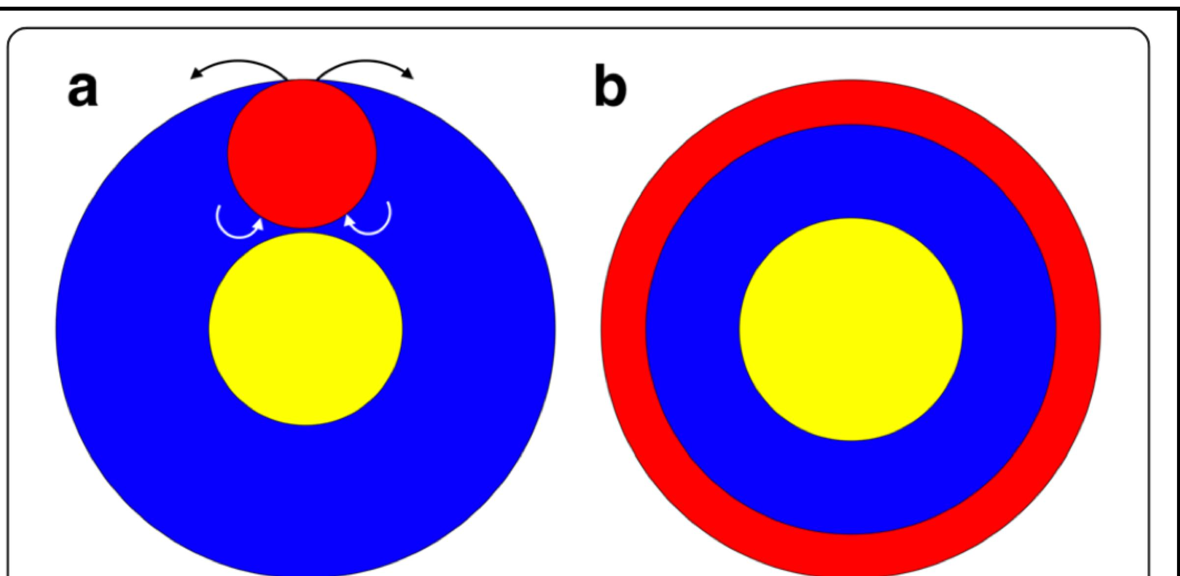
**Fig. 1** Isostatic readjustment and lateral spreading of an initially spherical impact-induced melt pool (**a**) leading to global magma ocean formation (**b**). Due to the lower density of the melt (red) compared to the surrounding solid mantle (blue), the solid mantle rises isostatically beneath the melt pool (white arrows) by solid-state deformation and the melt spreads over the surface of the planetary embryo (black arrows). The proto-core is shown in yellow
