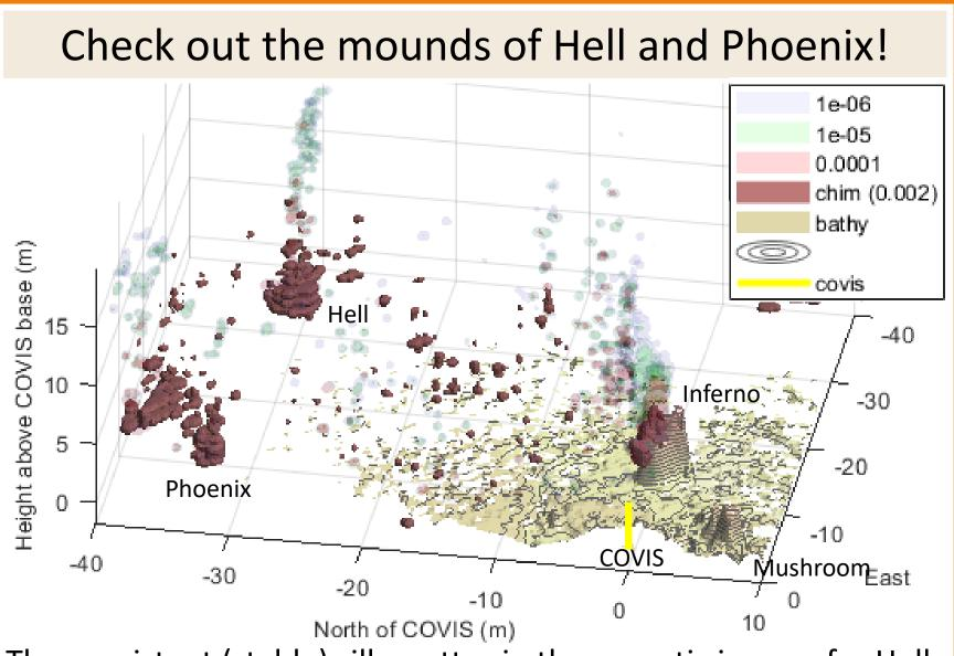
The consistent (stable) silhouettes in the acoustic images for Hell and Phoenix suggest we could get better bathymetry for the area with intelligent processing of the imaging data.
