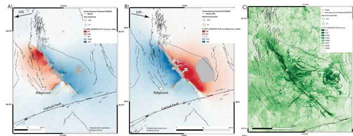
**Figure 2.** A) Sentinel-1 ascending track 64 pair 7/04-7/10 with non-standard 7 by 3 looks (averaging) and low filtering. Manual masking of main ruptures performed to improve phase unwrapping. B) Sentinel-1 descending track 71 pair 7/04-7/16 with similar processing. C) Coherence estimated before filtering and averaging. D) Advanced damage proxy map from coherence time series analysis of track 64 (O. Stephenson et al. poster on Monday).
