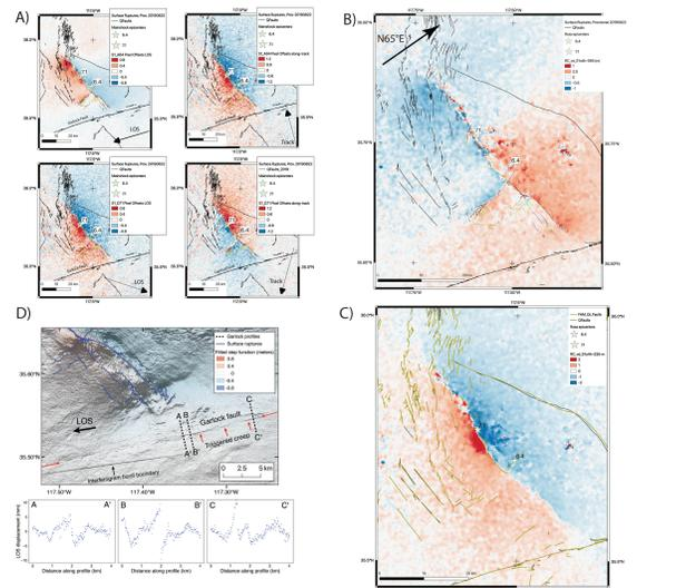
**Figure 4.** A) Original pixel offset maps from Sentinel-1 in range (line-of-sight) and azimuth (along-track) used for 3D computations. B) Horizontal motion in azimuth 65° highlights slip on Mw 6.4 ruptures. C) Horizontal motion in azimuth 335° shows very large strike-slip motion on Mw 7.1 rupture near epicenter. Same faults as in Fig. 3. D) Time-series step-function fit of coseismic deformation using MintPy [3] showing shallow triggered slip on Garlock Fault (from [4]).
