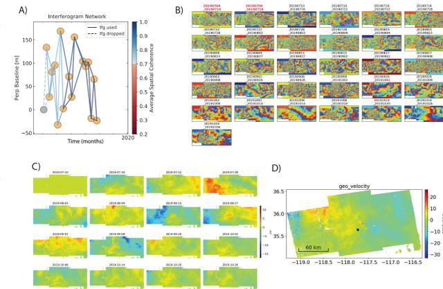
**Figure 5.** Postseismic time-series analysis with MintPy [3] for Sentinel-1 track A64 stack in radar coordinates through 10/26. A) Network of interferograms vs. time, coseismic pairs dropped from postseismic analysis. B) Interferograms rewrapped to original phase. C) Line-of-sight (LOS) displacements of post-seismic dates from SBAS inversion relative to 7/10 and reference point marked with square. D) Mean velocity fit to time series after geocoding. No atmospheric corrections applied yet.
