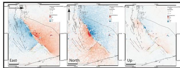
**Figure 3.** Three components (East, North, Up) of coseismic surface deformation calculated from SAR pixel offset tracking on Copernicus Sentinel-1 images acquired from tracks A64 and D71 (see Fig. 4A). A 500 meter median filter was applied to the offsets. Faults from USGS Qfaults and preliminary ruptures [5] overlain. Note higher noise level on north component due to larger along-track (azimuth) pixel size of Sentinel-1
