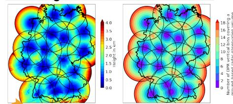
Radar network of DWD. Black circles are the maximum radar ranges. The heights of radar bin above ground in km (left). The number of GPM-DPR profile range bins contained within a single RADOLAN bin.
