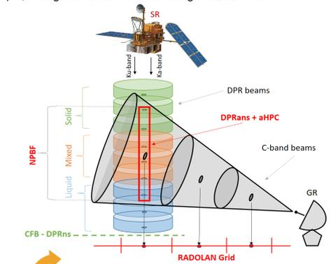
Schematic of a scan scenario by the ground radar and a DPR profile. Note the further the radar bin the more profiles DPR bins are covered by the ground radar.
