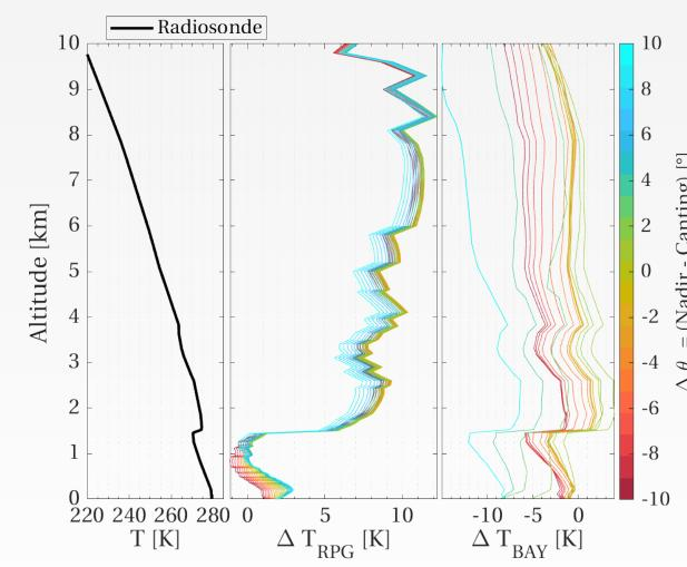
Additional uncertainties are introduced by observing brightness temperatures at different elevation angles. The data analysis must consider effects on retrievals due to wave-forcing off-set on elevation angles.
