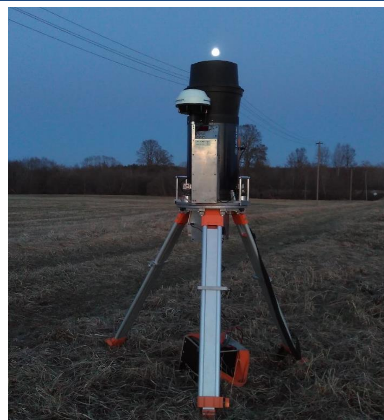
Fig. 1. The Digital Zenith Camera
