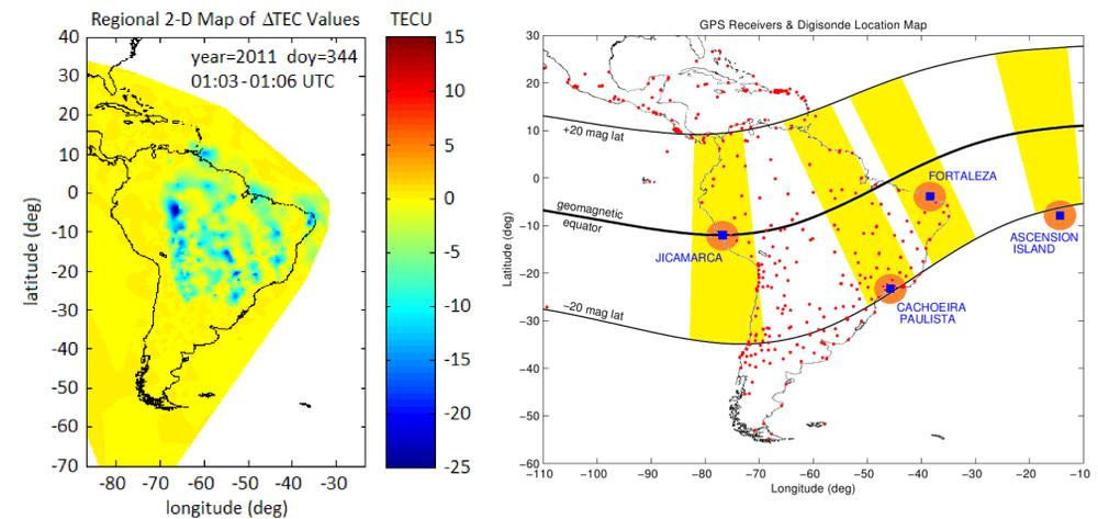
Left: 2-D  $\Delta$ TEC data map showing EPBs. Right: Map of ground-based GPS receivers and digisonde stations.
